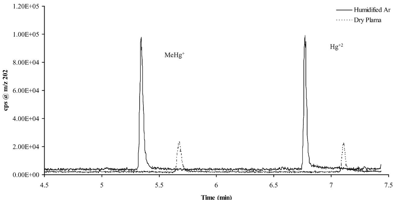
**Fig. 2** Chromatogram of ethylated mercury species from unspiked SRM 2977 extract obtained by SPME-GC-ICP-MS for both the humidified argon and dry plasma modes of operation (traces shifted for clarity).
