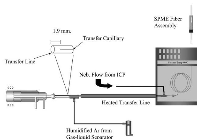
Fig. 1 Diagrammatic representation of the basic components of the SPME-GC-ICP-MS interface.
