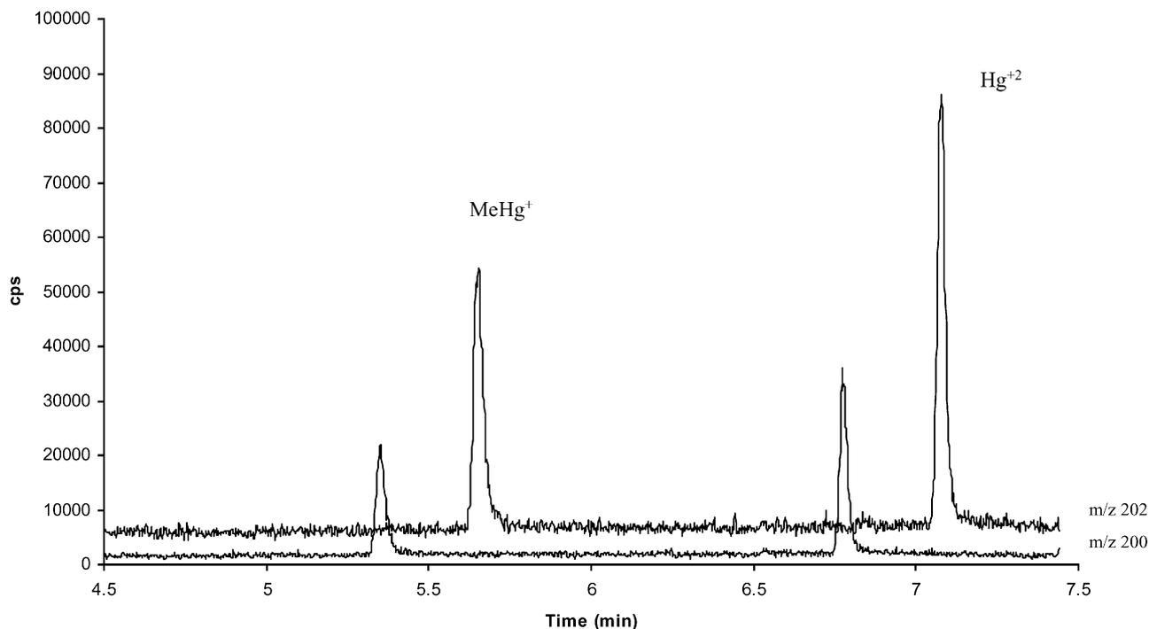
Fig. 3 Chromatogram of ethylated mercury species for unspiked SRM 1566b extract obtained by SPME-GC-ICP-MS (traces shifted for clarity).
