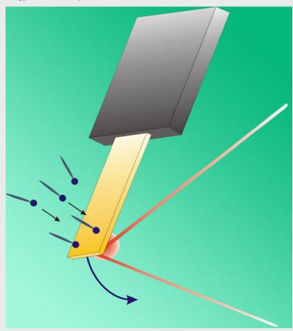
CSTL researchers measured the surface stress of a monolayer film on gold by measuring the changing curvature of a gold-coated glass cantilever as molecules of mercaptobenzoic acid were deposited on the gold. The change in curvature was detected by the shifting reflection of a laser beam impinging onto the back side of the glass.
