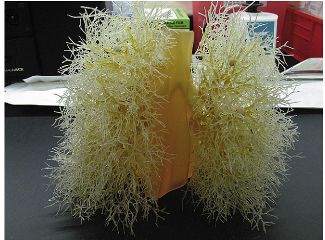
Figure 2. Photograph of the lung phantom being scanned by the Food and Drug Administration/National Institute of Biomedical Imaging and Bioengineering research team.
