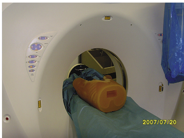
Figure 6. The same phantom used in 1A is used for the study of system-dependent measurement errors (part 1C). This inter-center comparison study aims to characterize sources of variability complementary to those of 1A, including intra-machine effects (such as reconstruction filter) and inter-machine variability (such as manufacturer, number of detector rows, and imaging center).
