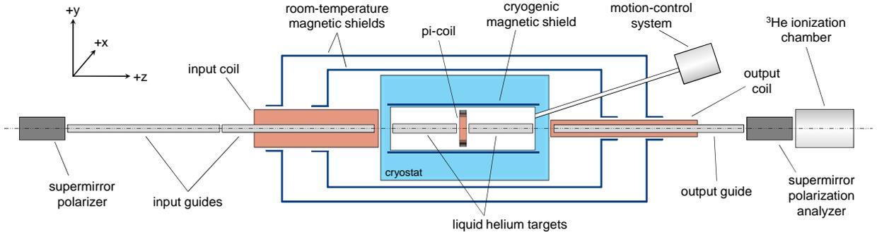
Figure 1: Schematic diagram of the neutron polarimeter apparatus for the Neutron Spin Rotation experiment.
