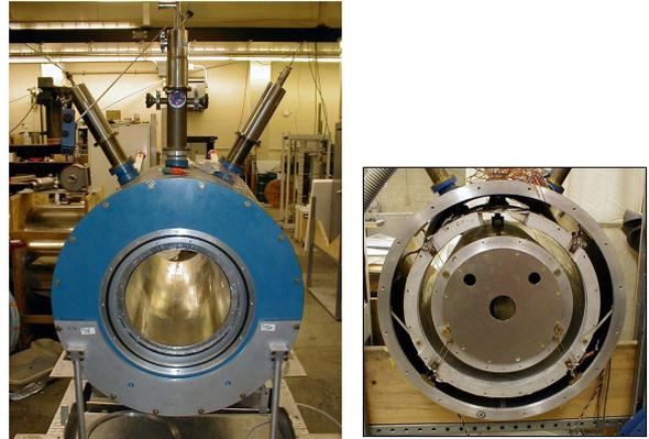
Figure 10: Photos of the cryostat. The outer 77-K vessel held liquid nitrogen and the inner 4-K vessel held liquid helium. The inside diameter of the 4-K vessel formed the cold bore and was lined with cryogenic mumetal magnetic shielding.
