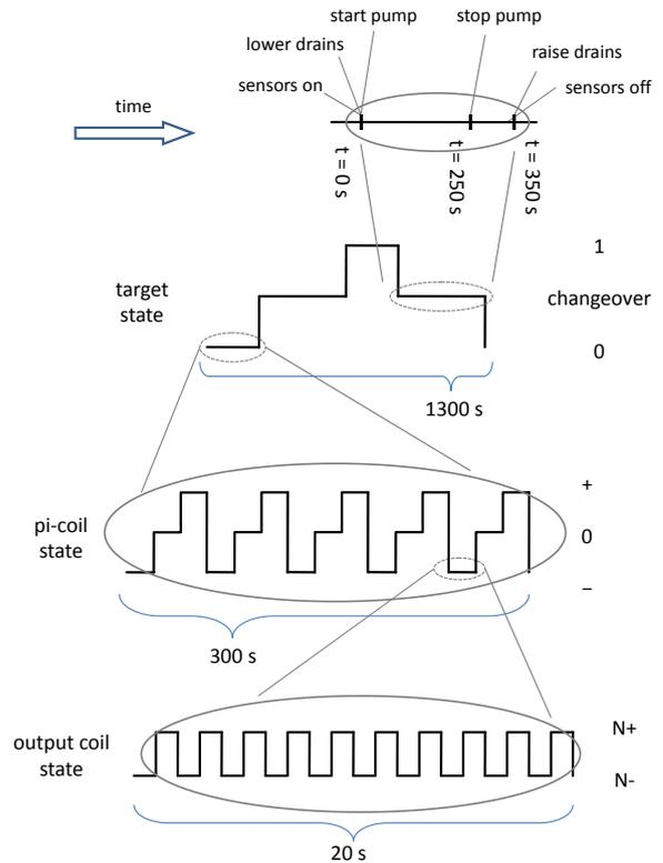
Figure 11: Diagram of the control sequence. The output coil is flipped at a rate of 1 Hz. Each pi-coil state has 10 output coil flips. Five pi-coil sequences make a target sequence. A target-change routine following each target state switched the liquid helium target between target states. Two consecutive target sequences constitute a target cycle.
