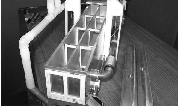
Figure 4: Layout of the neutron beam collimation within a target.  ${}^6\text{LiF}$ -plastic was glued onto aluminum backing frames and then glued into the target chambers. The size and spacing of the collimation was chosen to prevent neutrons with wavelengths larger than 2 nm from reflecting off a chamber wall and then being accepted into the  ${}^3\text{He}$  ionization chamber. Additional  ${}^6\text{LiF}$ -plastic was glued onto the upstream face of the targets.
