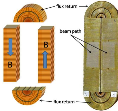
Figure 5: Diagram of the pi-coil. The coil is wound so that the left and right solenoids produce vertical magnetic fields through the region of the passing neutron beam. These fields are oriented opposite to each other, and the curved solenoid sections on top and bottom provide flux return for both coils.
