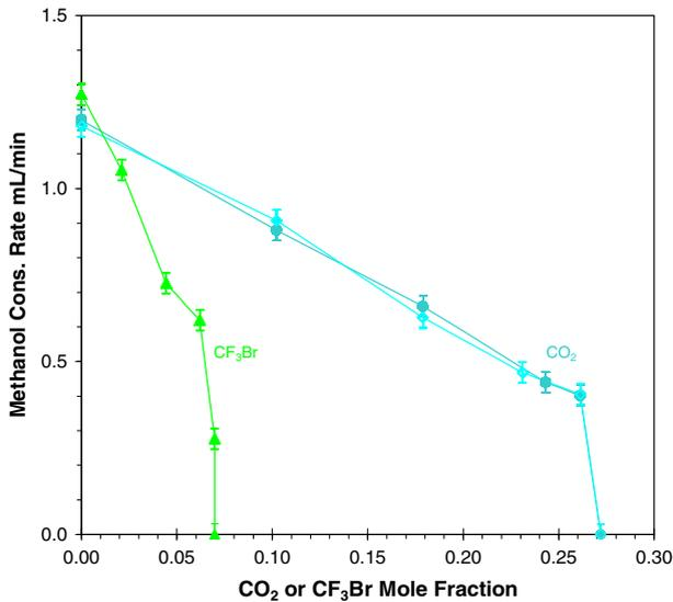
**Figure 11. Cup burner methanol consumption rate as a function of CO<sub>2</sub> and CF<sub>3</sub>Br volume fraction in air.**
