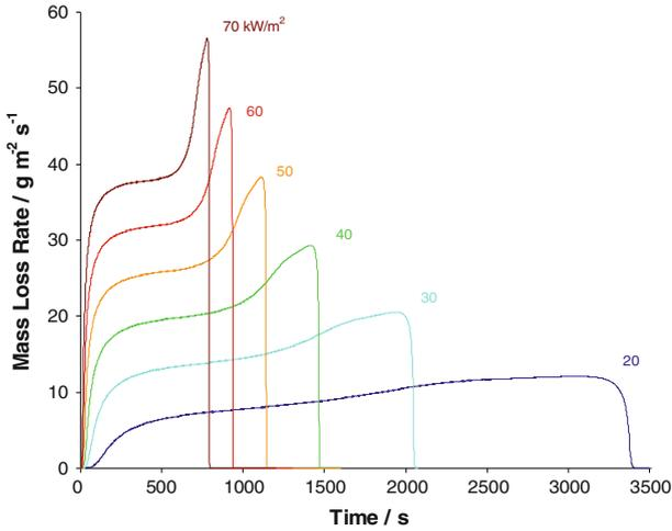
**Figure 2. Calculated mass loss rate of 25.4 mm thick PMMA as a function of time for incident external flux rates of (10, 20, 30, 40, 50, 60, and 70) kW/m<sup>2</sup>.**
