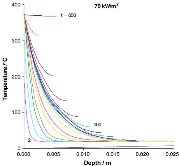
**Figure 5. 1-D temperature profile through PMMA slab (initially 25.4 mm thick) as a function of time (indicated on curves), at incident flux or 70 kW/m<sup>2</sup>.**
