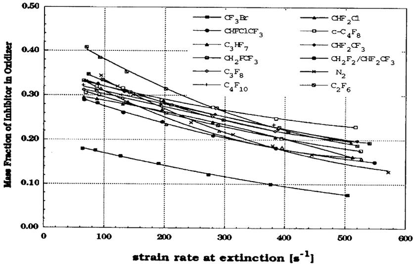
**Figure 7. Mass fraction of inhibitor in the oxidizer flow (air) necessary to extinguish a counterflow diffusion flame over heptane, as a function of strain rate ( $T_{\text{air, inlet}} = 150^\circ\text{C}$ ).**
