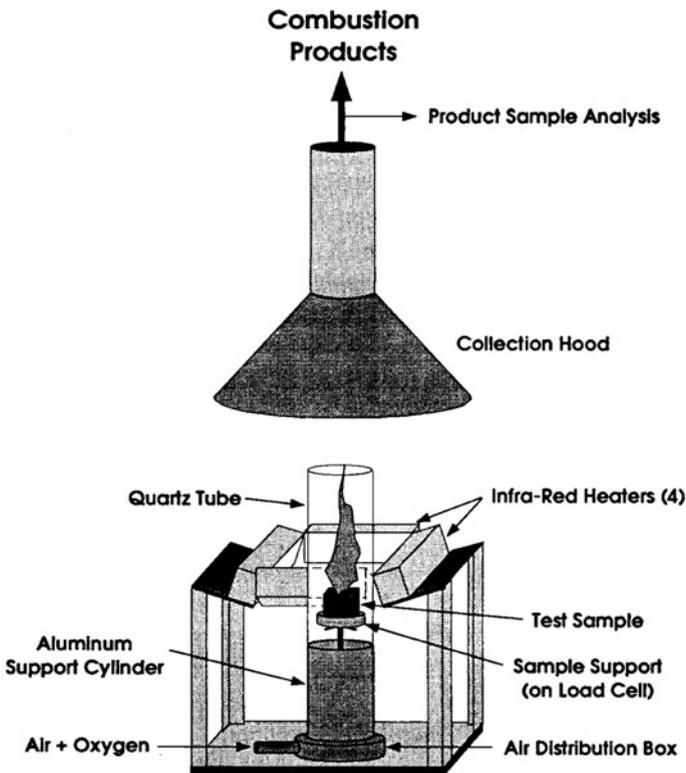
**Figure 24. FM Global flammability apparatus (50 kW scale) [52].**
