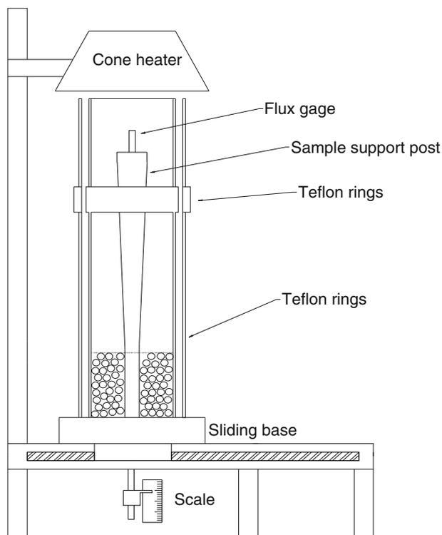
**Figure 25. Radiantly Enhanced Extinguishing Device (REED) [11].**
