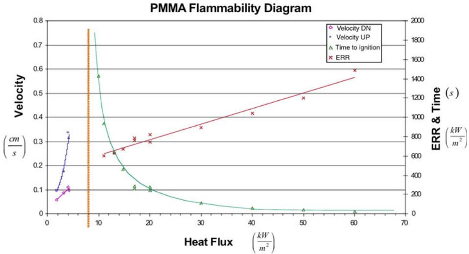
**Figure 14. Flammability diagram for PMMA (from Ref. [49]; used with permission of the author).**
