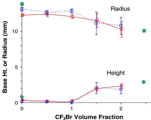
**Figure 12. Flame height and radius for methane-air cup-burner flames with CF<sub>3</sub>Br added to the air stream at increasing volume fraction [44].**
