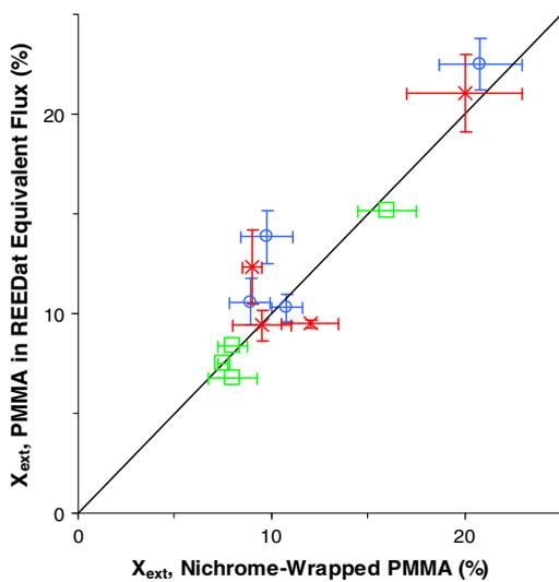
**Figure 21. Agent (HFC-23, HFC-227ea, FC-2-1-8, and FC-3-1-10) extinguishing volume fraction for PMMA with Nichrome wire heating, or at an equivalent heat flux achieved in the REED device (○: Ref. [57]; □ and +: 48 W and 192 W cases of Ref. [9]).**
