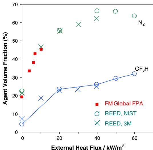
**Figure 23. HFC-23 or N<sub>2</sub> volume fraction for extinguishment of PMMA in the REED device as a function of external heat flux (NIST and 3M results are given). Tests with N<sub>2</sub> extinguishing PMMA in the FM Global FPA [17] are also shown.**
