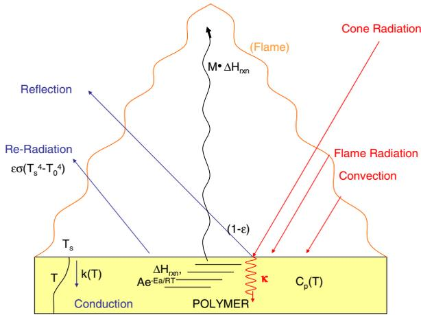
**Figure 1. Heat flows at the surface of a burning thermoplastic polymer, with some of the processes in the condensed phase illustrated also.**
