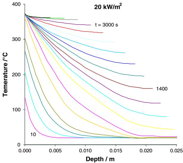
**Figure 4. 1-D temperature profile through PMMA slab (initially 25.4 mm thick) as a function of time (indicated on curves), at incident flux or 20 kW/m<sup>2</sup>.**
