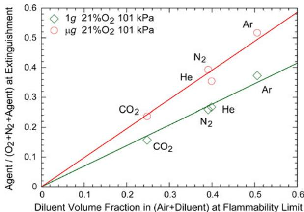
**Figure 8. Correlations between the cup burner extinguishment limits and the critical flammability limits expressed in terms of the agent volume fractions in oxidizer, from [27] for a methane-air flame.**
