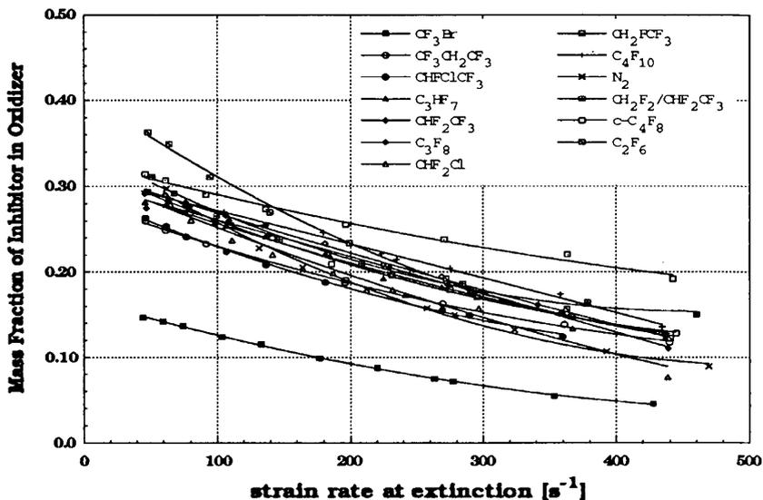
**Figure 6. Mass fraction of inhibitor in the oxidizer flow (air) necessary to extinguish a counterflow diffusion flame over heptane, as a function of strain rate ( $T_{\text{air, inlet}} = 25^{\circ}\text{C}$ ).**
