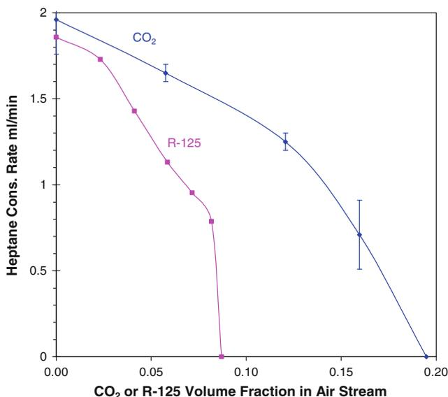
**Figure 10. Cup burner heptane consumption rate as a function of CO<sub>2</sub> or R-125 volume fraction in air.**
