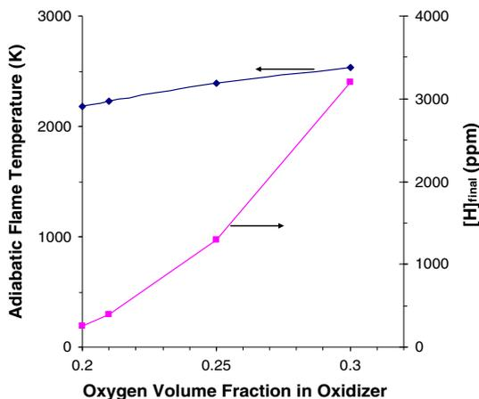
**Figure 9. Adiabatic flame temperature and final H-atom volume fraction as a function of oxygen volume fraction in the oxidizer in a  $\text{CH}_4/\text{O}_2/\text{N}_2$  premixed flame.**
