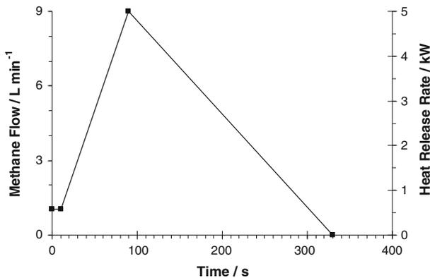
**Figure 20. Input power versus time for NEBS fire test [71].**
