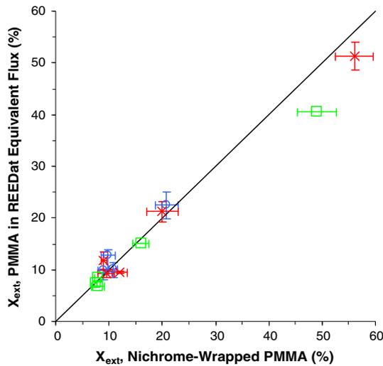
**Figure 22. Agent extinguishing volume fraction with the agents in Fig. 21 as well as with IG-541 for PMMA with Nichrome wire heating, or at an equivalent heat flux achieved in the REED device (○: Ref. [57]; □ and +: 48 W and 192 W cases of Ref. [9]).**
