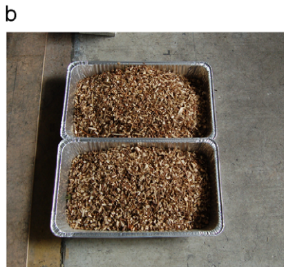
Fig. 2. (a) Digital pictures of Norway Spruce trees used to produce mulch for firebrand generator; details of the tree are shown. (b) Mulch that is produced and used per experiment (2.8 kg).
