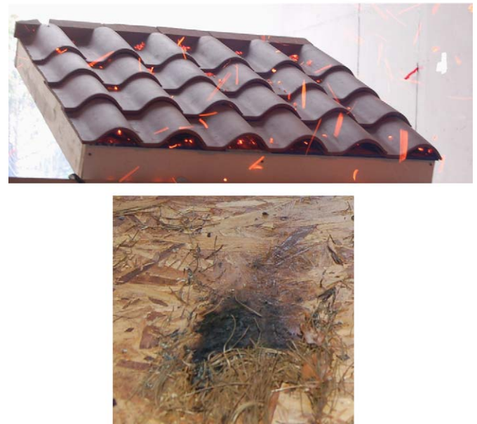
Fig. 9. Images of experiments conducted using OSB/CT without bird stops installed. Dried needles and leaves have been inserted under the tiles. Intense SI was observed within the OSB base layer and eventually FI was observed.
