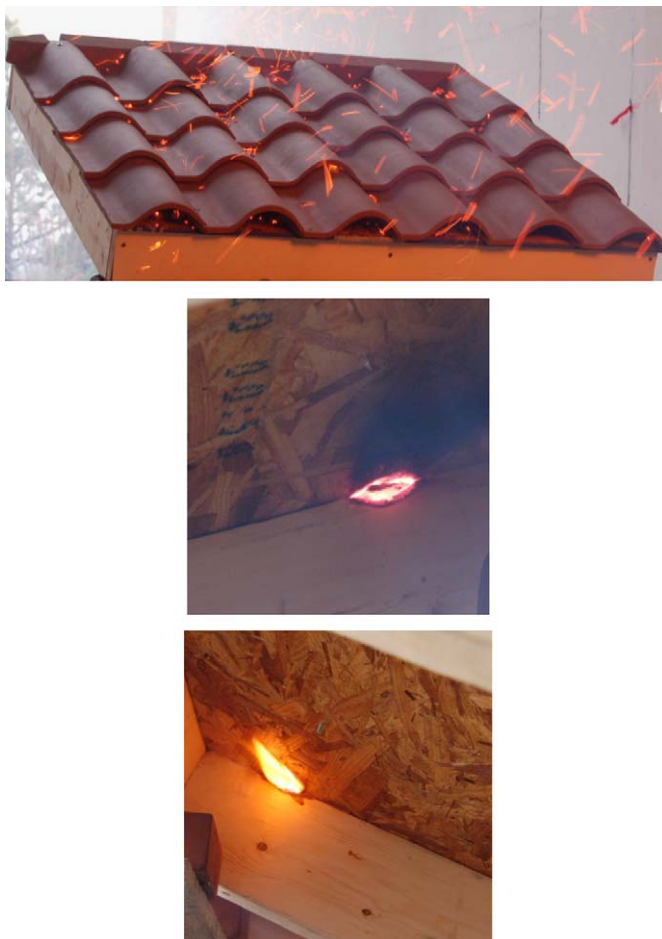
Fig. 6. Images of experiments conducted using OSB/CT without bird stops installed. Intense SI was observed within the OSB base layer and eventually FI was observed.
