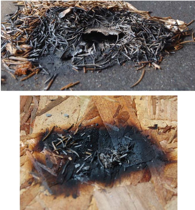
Fig. 10. Images of experiments conducted using OSB/TP/CT with bird stops installed. Dried needles and leaves have been inserted under the tiles. SI was observed within the OSB base layer.
