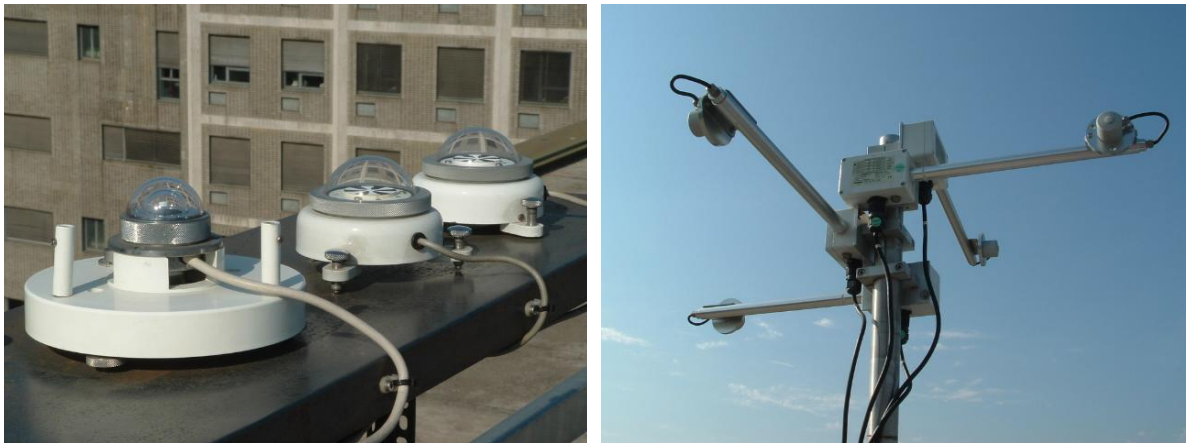
Figure 1 and 2. MeteoLAB . Instruments for global radiation and photometric measurement.
