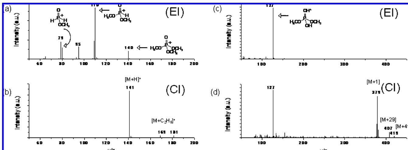
**Figure 4.** Electron impact (EI) and chemical ionization (CI) spectra of trimethyl phosphate (a, b) and long-chain alkyl phosphate (c, d). A.U. denotes arbitrary units of intensity.
