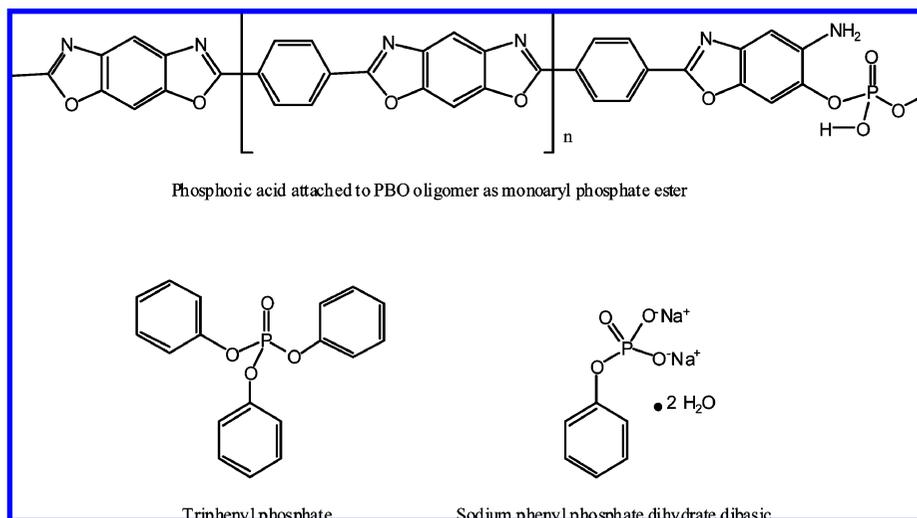
**Figure 5.** Chemical structure representation of phosphoric acid chemically bound to PBO oligomer as a monoaryl phosphate ester. To underscore the stability of the monoaryl phosphate ester bond, the chemical structures of triphenyl phosphate (a triaryl phosphate ester) and sodium phenyl phosphate dibasic dihydrate (a monoaryl phosphate ester), which are available commercially, are also shown.
