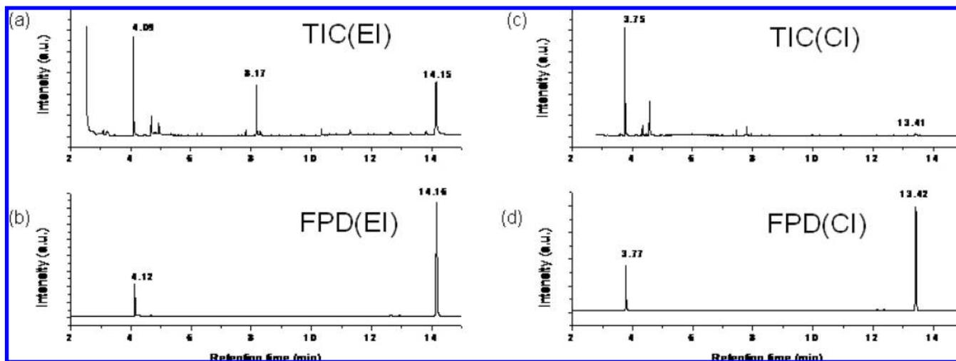
**Figure 3.** Total ion current (TIC) chromatograms (a) and (c) and parallel flame photometric detector (FPD) chromatograms (b, d) of methylated aqueous extract from PBO fibers under electron impact (EI) (a, b) and chemical ionization (CI) (c, d) test conditions. A.U. denotes arbitrary units of intensity.
