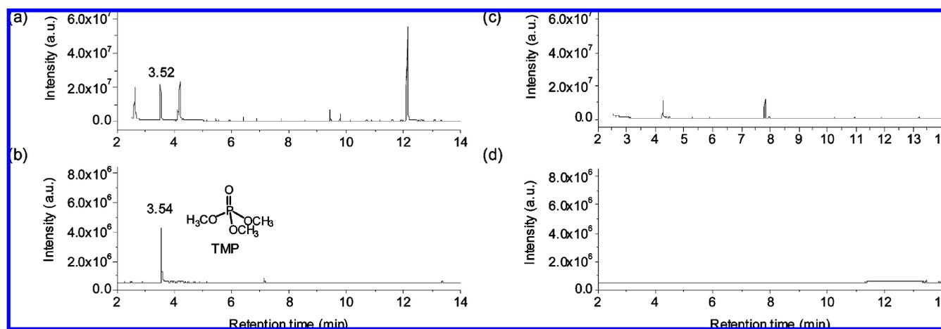
**Figure 8.** (a) Total ion chromatography (TIC) and (b) FPD spectrum of UV-exposed 2nd Caustic treated 1st PBO fiber Solution in the EI mode of GC/MS. (c) TIC and (d) FPD spectrum of UV-exposed water blank in the EI mode of GC/MS. A. U. denotes arbitrary units of intensity.
