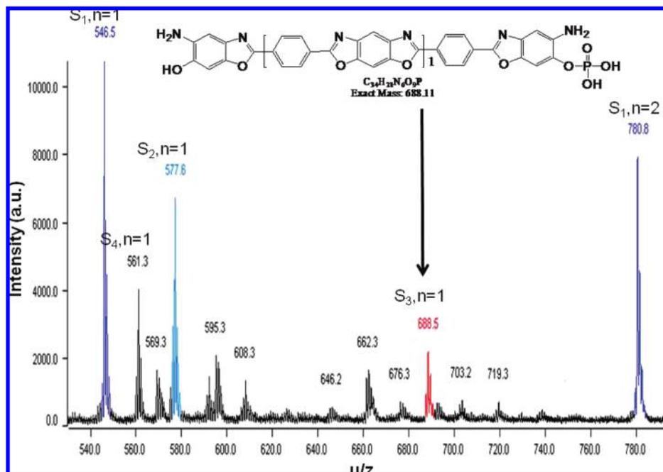
**Figure 6.** MALDI-TOF MS of low molecular mass model PBO oligomers. A.U. denotes arbitrary units of intensity.
