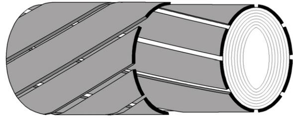
**Figure 4.** Schematic of a multi-layer cable, showing how each layer is configured out of multiple conductors.
