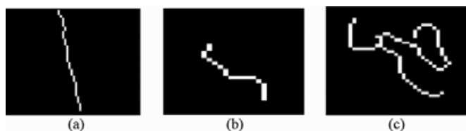
FIG. 4—Three entity examples existing in the primary edge image. (a) represents a striation mark, or bullet signature; (b) and (c) do not.
