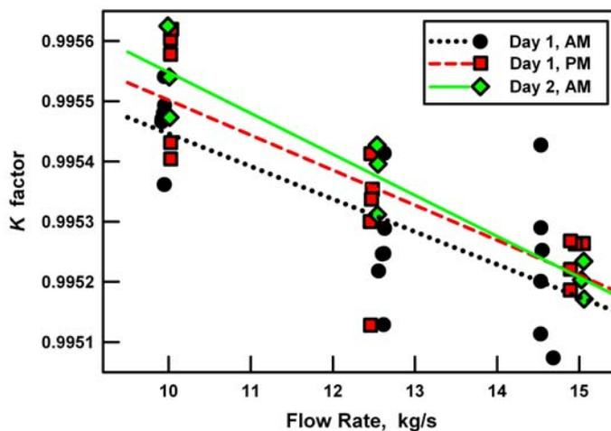
**Figure 4. Calibration of electromagnetic flow meter.**
