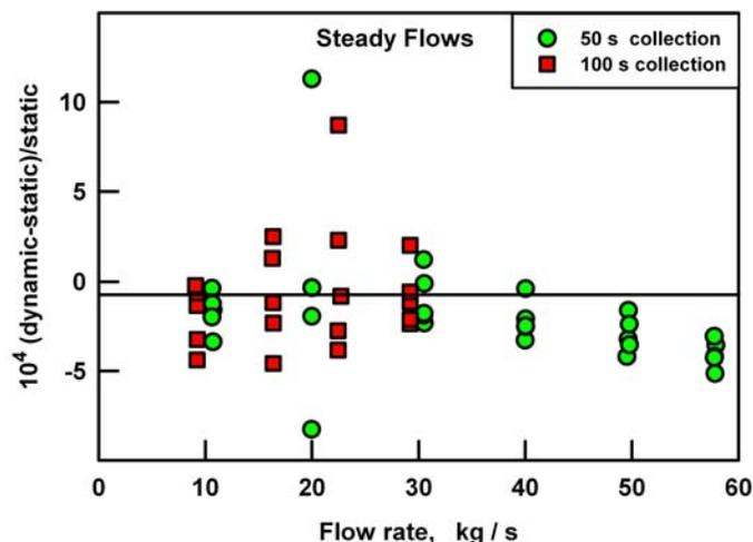
**Figure 3. Fractional differences between dynamic measurements and NIST's static gravimetric standard for steady flows from [2].**
