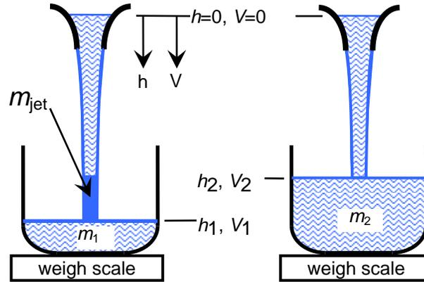
Figure 2. Schematic diagram of a dynamic calibration system at two times,  $t_1$  and  $t_2$ .
