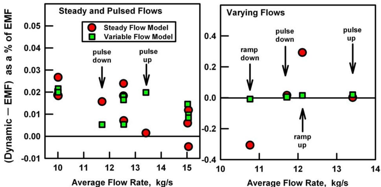
**Figure 7. Comparisons of dynamic flow measurement and calibrated EMF. The variable flow model [Eq. (10)] was implemented numerically using Eqs. (12) - (14). For the steady flow model,  $h \equiv 0$  in Eq. (13). Note: the scale on the left panel is 14× finer than the scale on the right panel.**
