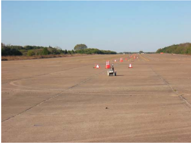
Fig. 4. Line-of-sight course set up over a 1 km distance on an airstrip with orange safety cones marking test points.
