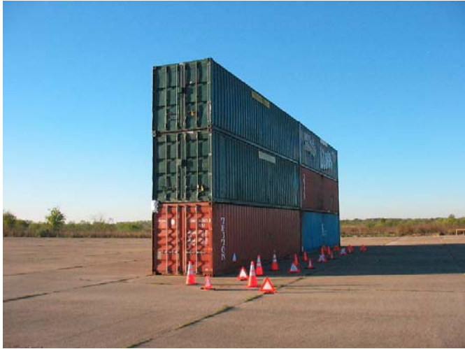
Fig. 8. The far side of the container stack showing placement of the final (500 m) figure-eight LOS test station and subsequent NLOS test points located along the back wall.
