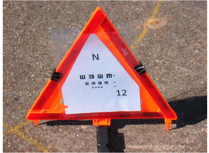
Fig. 6. Example of a visual acuity chart used at each test station for both the LOS and NLOS methods
