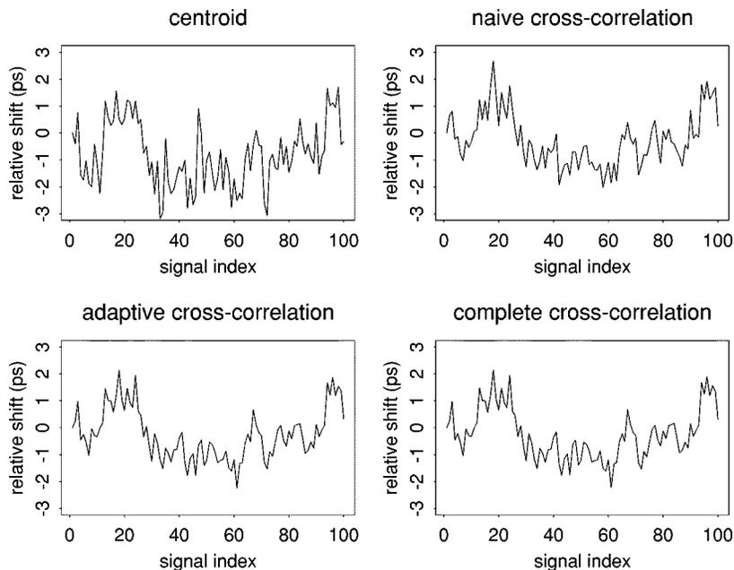
Fig. 6. Relative shift estimates for experimental data due to different methods.
