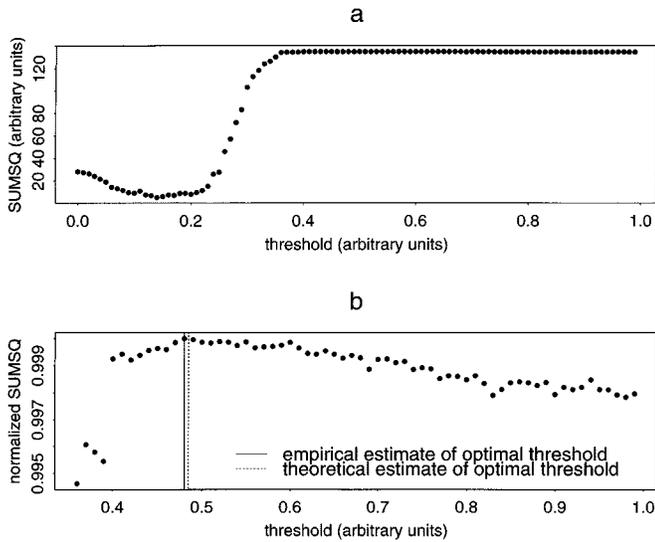
Fig. 3. (a): Total power ( $SUMSQ$ ) of the average of 100 realizations of  $g$  where  $\sigma_{jit} = 3$ ,  $\sigma_{add} = 0.08$  and  $\sigma_{shift} = 5$ . (b): Normalized  $SUMSQ$  for the same case.
