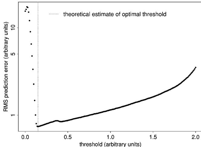
Fig. 2. RMS prediction error for centroid estimate of relative shift of noisy realizations of  $g$  where  $\sigma_{jit} = 2.5$ ,  $\sigma_{add} = 0.02$  and  $\sigma_{shift} = 5$ .
