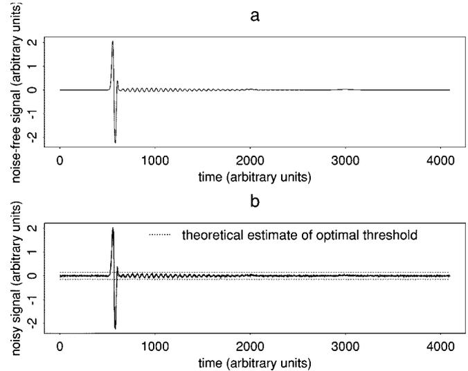
Fig. 1. (a): Noise-free simulated signal. (b): Noisy simulated signal where  $\sigma_{add} = 0.02$  and  $\sigma_{jit} = 2.5$ . We plot the  $\pm \hat{\alpha}$  where  $\hat{\alpha}$  is the optimal threshold for the centroid method.
