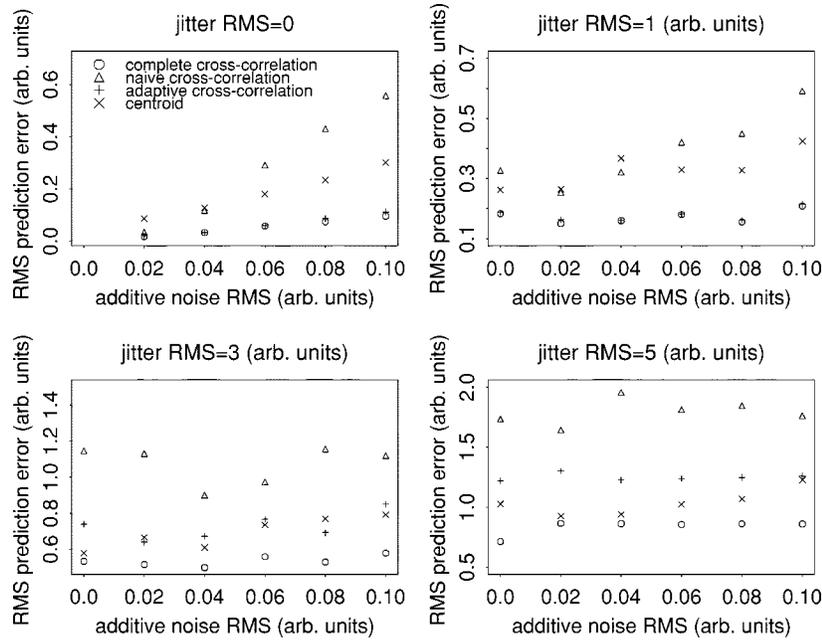
Fig. 4. RMS prediction error versus RMS additive noise when 100 misaligned simulated signals are aligned by different methods.
