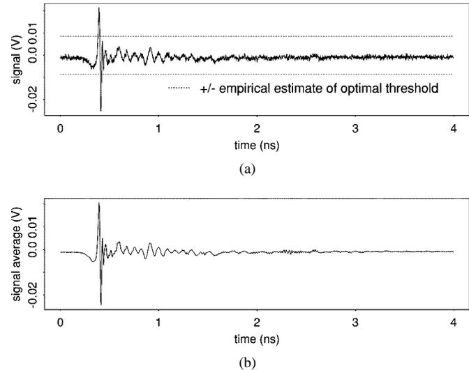
Fig. 5. (a) Measured oscilloscope signal. (b) Average of 100 aligned oscilloscope signals using cross-correlation method estimates of relative shifts. The interval between samples is = 1.953 ps.
