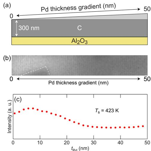
FIG. 2. (Color online) (a) A cross-sectional schematic and (b) a top view IR image of a Pd/C bilayer thickness gradient sample at 423 K deposited on an Al<sub>2</sub>O<sub>3</sub> (0001) substrate. (c) 29 raw IR intensities as a function of the Pd thickness ( $t_{Pd}$ ).
