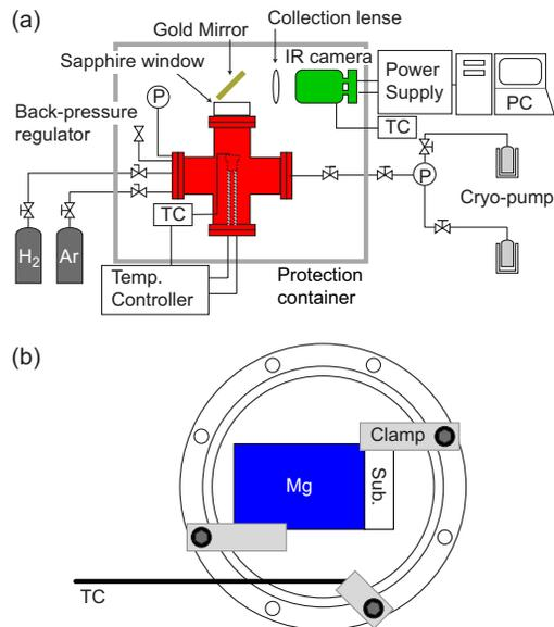
FIG. 1. (Color online) (a) A top view diagram of the IR imaging setup. The reaction chamber with the heating stage and the IR camera are in red and green, respectively. TC, P, and PC denote the *k*-type thermocouple, the pressure gauge, and the personal computer, respectively. (b) A top view diagram of the heating stage.
