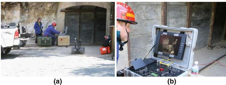
**Fig. 9.10** (a) Robot operator positioned at the entrance to the Hazel-Atlas mine tunnel. (b) The robot was operated in a non-line-of-sight condition more than 100 m inside the tunnel
