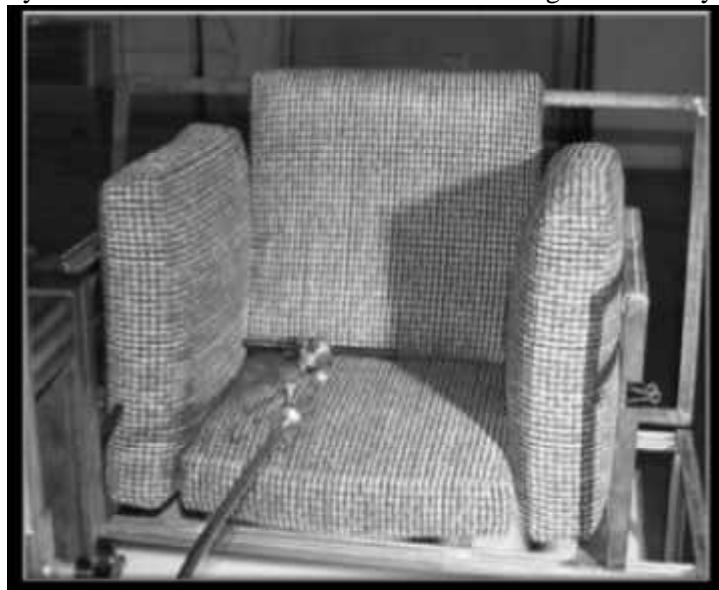
Figure 1. Four cushion mock-up in Cal 133 mock-up frame, showing placement of Tee burner igniter. The heat release rate properties of these mock-ups were measured using standard oxygen consumption calorimetry in a 2 meter furniture calorimeter in the large-fire facility at NIST.
