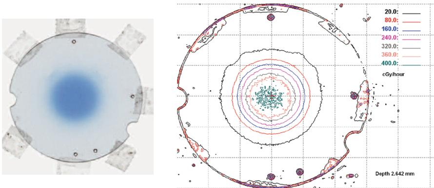
**Figure 23-15.** EBT-1 film exposed at a distance 2.642 mm from the inner surface of a CCX plaque and the dose rate distribution calculated from the film using MSKCC’s Contour film dosimetry program.
