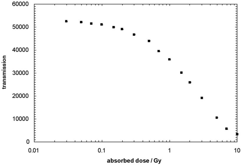
**Figure 23-4.** Calibration curve for EBT film read in the red channel of an uncorrected photo-scanner curve from data in table 23-5.
