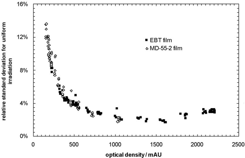
**Figure 23-6.** A characteristic curve for a laser densitometer. The relative standard deviation on the y-axis refers to the standard deviation of the average of the optical densities of the pixels of uniformly irradiated films.
