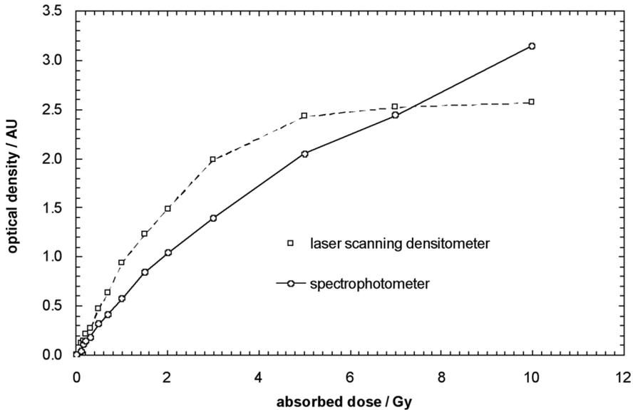
**Figure 23-8.** Comparison of linearity between a spectrophotometer and a laser scanner for reading EBT film.
