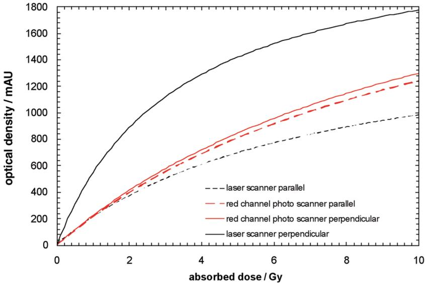
**Figure 23-9.** Effect of EBT film orientation relative to coating direction in two scanners.
