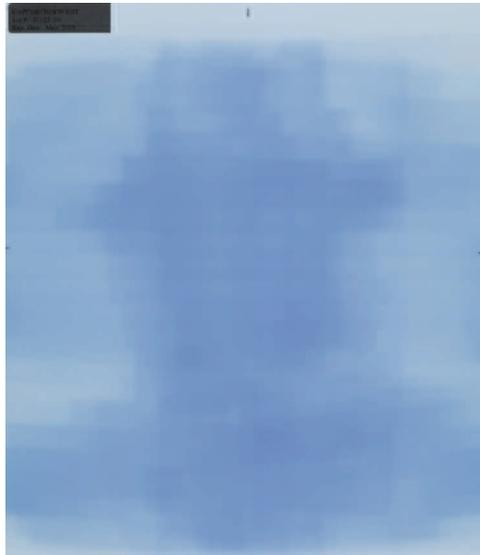
**Figure 23-10.** GAFCHROMIC EBT film exposed to a full head and neck IMRT treatment in the coronal plane of a phantom. The film shows the fiducial marks at the crosshairs, and a label of the film lot placed at the initially marked upper left corner.
