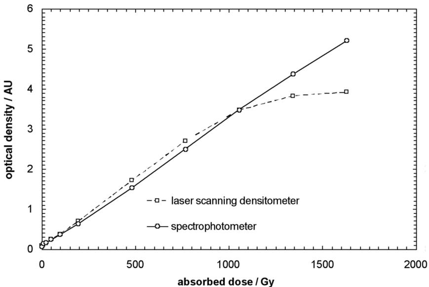
**Figure 23-7.** Comparison of linearity between a spectrophotometer and a laser scanner for reading HD-810 film.
