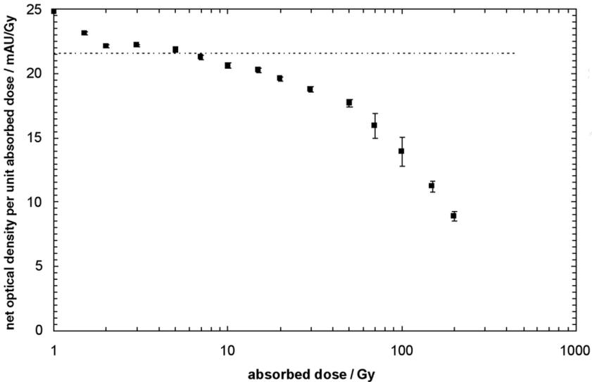
**Figure 23-3.** Net optical density per unit absorbed dose to water medium curve for MD-55-2 film read at 633 nm from data in table 23-4. The dashed line indicates the region of linearity between 5 Gy and 20 Gy.
