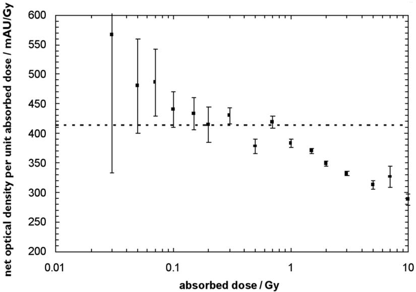
**Figure 23-5.** Net optical density per unit absorbed dose to water medium curve from data in table 23-5. The dashed line indicates a region of assumed linearity.
