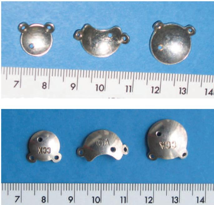
**Figure 23-13.** Front and back views of three types of  $^{106}\text{Ru}/^{106}\text{Rh}$  eye plaques (from left: CCA, CIA, and CCX types). These are “dummy” plaques, which are an exact silver replica of the appropriate plaque, but without the radioactive layer. They can be distinguished from the real plaque by the hole through the plaque and missing serial number.
