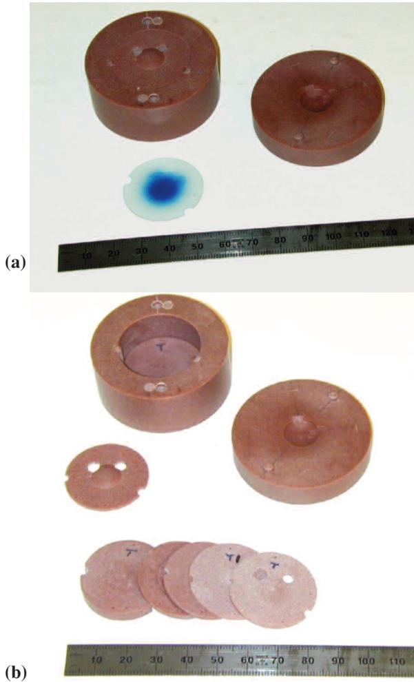
**Figure 23-14.** Pictures of the Solid Water™ eye phantom, which enables exact co-registration between the film and the plaque. The GAFCHROMIC film is placed between inserts of the phantom. (a) Assembled phantom with removed cover part and an exposed MD-55-2 film. (b) Body of the phantom and its various inserts.
