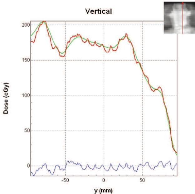
**Figure 23-12.** Vertical profiles through the dose distributions of the superimposed film and plan in figure 23-11 represented in absolute dose. The green line is the plan dose, the red line is the film dose, the blue line shows the difference between plan and film doses. The thumbnail picture in the upper left corner shows the location of the profile in the film plane. (FilmQA film dosimetry program).
