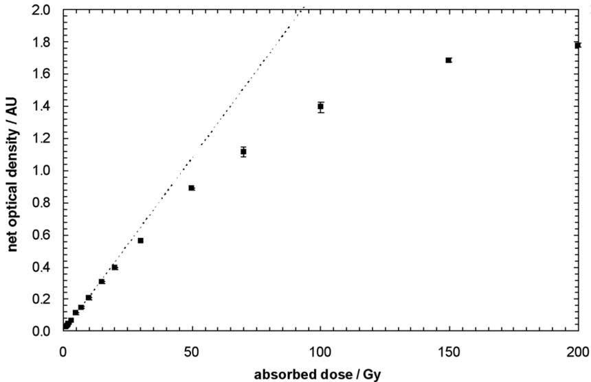
**Figure 23-2.** Calibration curve for MD-55-2 film read at 633 nm from data in table 23-4. The dashed line indicates the region of linearity between 5 Gy and 20 Gy.
