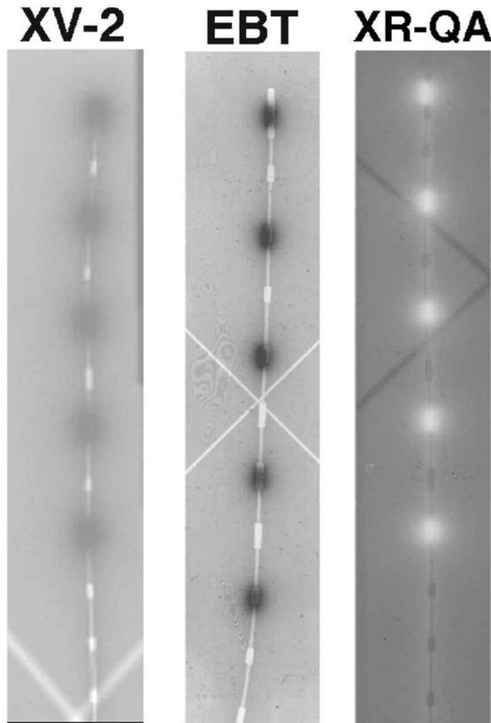
**Figure 23-16.** Examples comparing the use of photographic film (XV-2) with various radiochromic film models for QA measurements of HDR source positioning.
