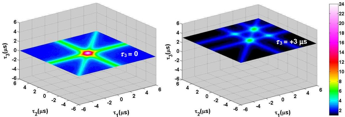
Fig. 2 Slices of  $g^{(4)}(\tau_1, \tau_2, \tau_3)$  data from the pseudo-thermal source for two fixed  $\tau_3$  delays, with color indicating measured value of  $g^{(4)}$ .
