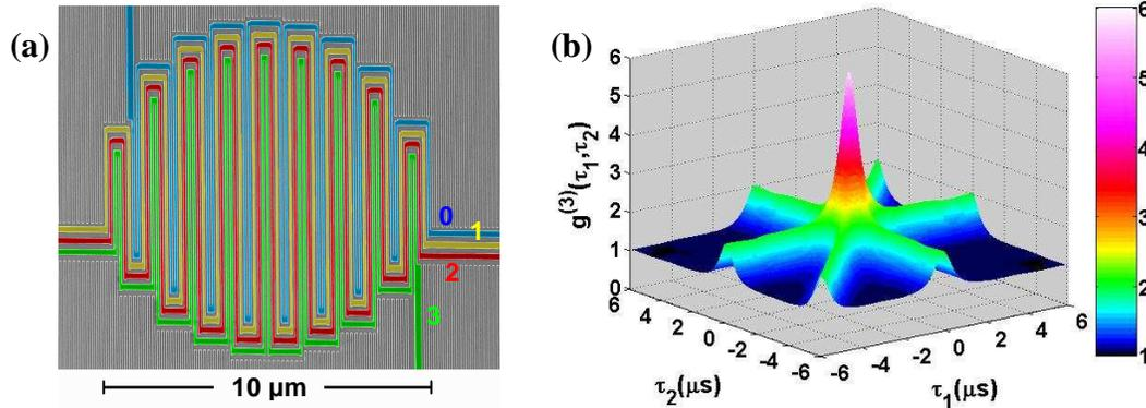
Fig. 1 (a) Scanning electron microscope image of four-element SNSPD, with nanowire elements 0-3 traced out in color. (b) Third-order coherence data from pseudo-thermal source, where both color and height indicate measured value of  $g^{(3)}$ .
