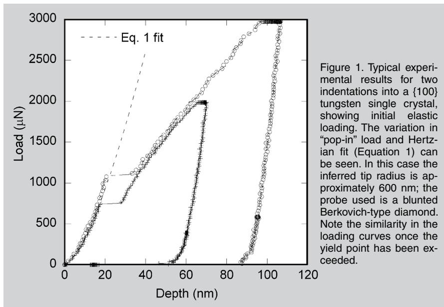
Figure 1. Typical experimental results for two indentations into a {100} tungsten single crystal, showing initial elastic loading. The variation in “pop-in” load and Hertzian fit (Equation 1) can be seen. In this case the inferred tip radius is approximately 600 nm; the probe used is a blunted Berkovich-type diamond. Note the similarity in the loading curves once the yield point has been exceeded.
