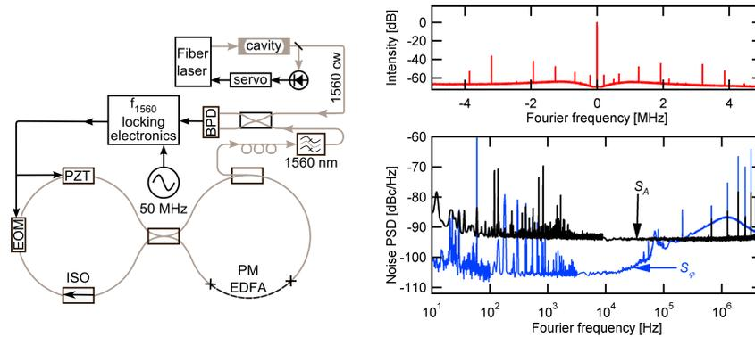
Fig. 1: Left: schematic of the comb (the CEO locking branch is not shown); BPD: balanced photodetector, ISO: isolator. Right: normalized spectrum (shifted by -50 MHz, top) as well as phase ( $S_\phi$ ) and amplitude ( $S_A$ ) noise power spectral density (PSD) (bottom) of the optical lock beat  $f_{1560}$ .
