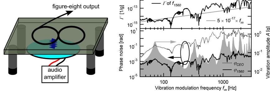
Fig. 2: Left: schematic of the shaking experiment. The laser actually covers the complete breadboard surface. Right: phase noise of the optical and CEO locks under vibration and average vibration amplitude on the breadboard (bottom); vibration sensitivity  $\Gamma$  of the optical lock (top).
