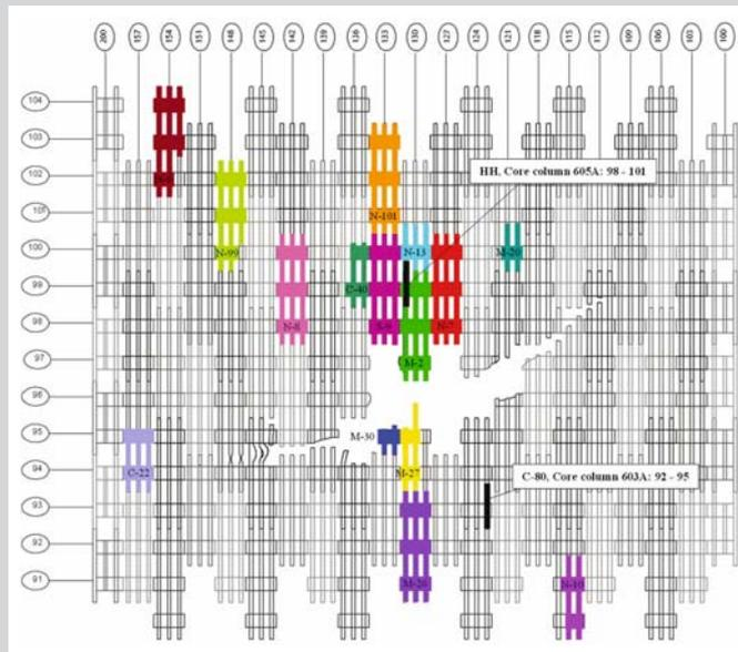
Figure 1. The locations of the recovered exterior wall columns surrounding the aircraft impact hole in WTC 1.
