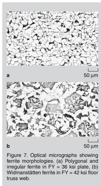
Figure 7. Optical micrographs showing ferrite morphologies. (a) Polygonal and irregular ferrite in FY = 36 ksi plate, (b) Widmanstätten ferrite in FY = 42 ksi floor truss web.
