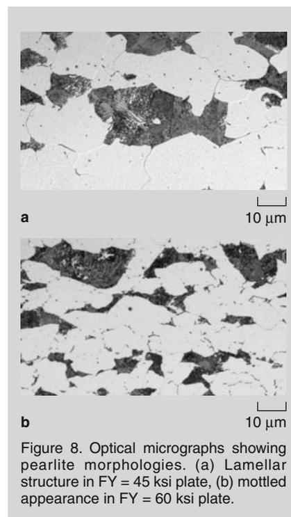
Figure 8. Optical micrographs showing pearlite morphologies. (a) Lamellar structure in FY = 45 ksi plate, (b) mottled appearance in FY = 60 ksi plate.
