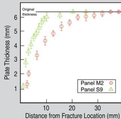
Figure 4. The thickness of exterior wall column plates near their fracture surfaces. Sections are from recovered columns M2 and S9 (see Figure 1), which were struck by the aircraft. Extensive necking demonstrates ductility even at high strain rate.
