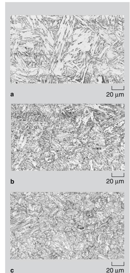
Figure 10. Optical micrographs showing structures of quench-and-tempered plates. (a) Widmanstätten or bainitic structure in  $FY = 70$  ksi plate, (b) tempered martensite in  $FY = 75$  ksi plate, and (c) tempered martensite in  $FY = 100$  ksi plate.
