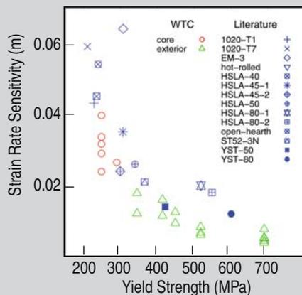
Figure 3. Strain rate sensitivities of the yield strength of core- and exterior wall-column steels compared to literature data on structural steel.
