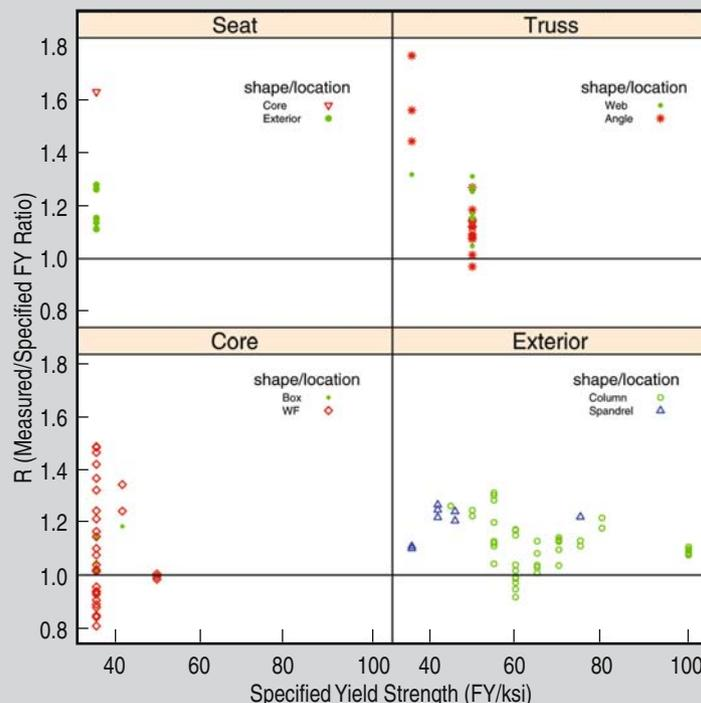
Figure 2. The ratio, R, of the measured yield strength to the specified yield as a function of specified yield strength for the 123 room-temperature tension tests.
