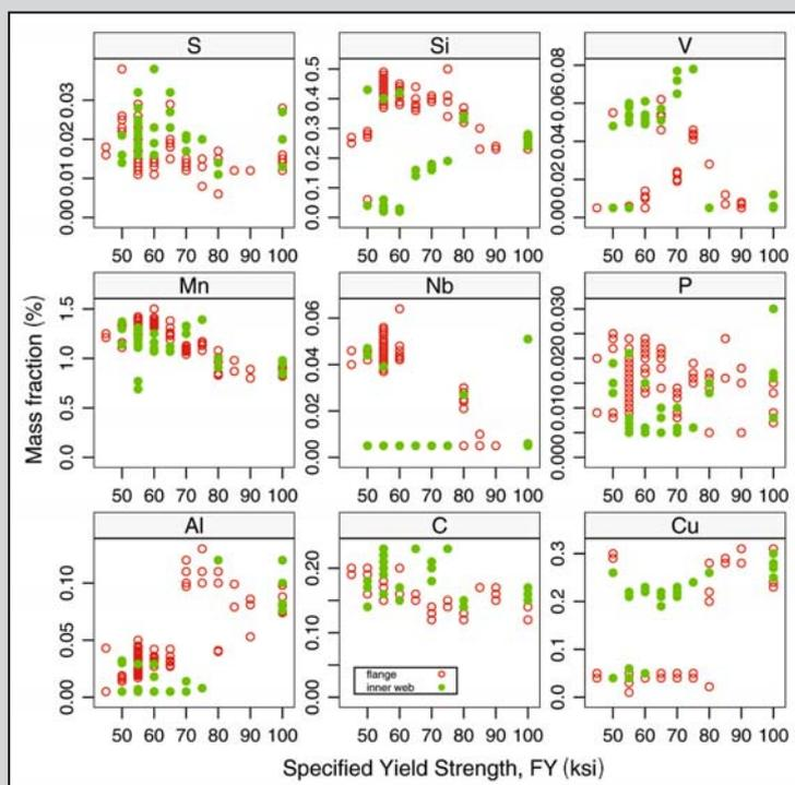
Figure 6. The chemical composition of exterior wall columns.
