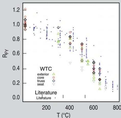
Figure 5. The high-temperature yield strength, normalized to the room-temperature value, of WTC steels compared to literature data for structural steels.
