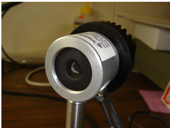
Figure 1. A temperature-controlled pyroelectric transfer-standard radiometer head 1 .
