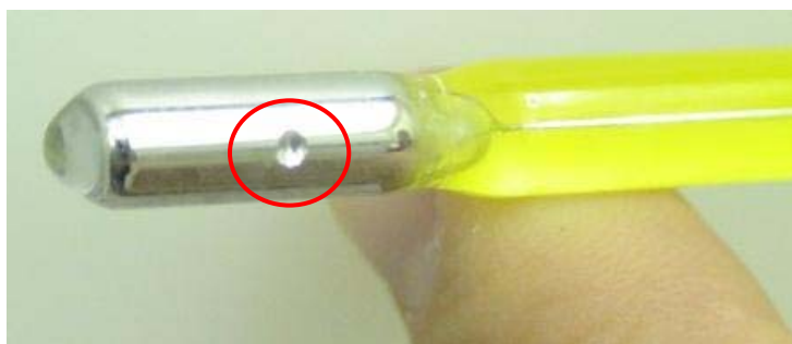
Fig. 7. Example of a gas bubble being washed out of the mercury in the thermometer bulb. The red circle indicates the gas bubble.
