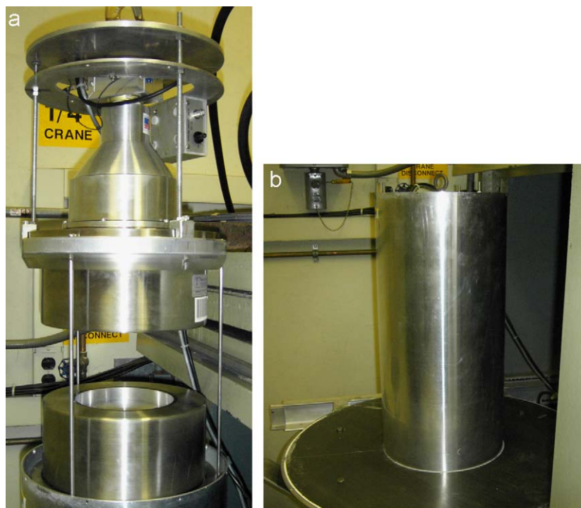
Fig. 3. The NIST NaI(Tl) coincident detector (a) open and (b) closed.
