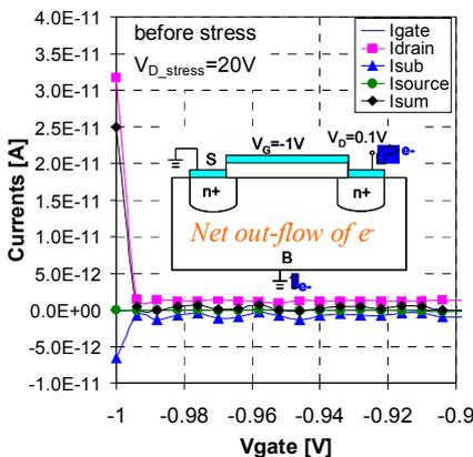
Fig. 4(a) Measurement of all the currents before stress for high-drain-voltage stress condition. The net current shows an out-flow of electrons.
