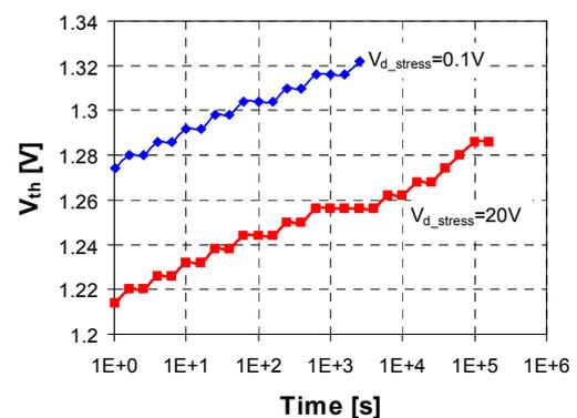
Fig. 1  $V_{TH}$  shifts as stress time increases at two stress conditions. ( $V_G=20\text{V}$ ,  $V_D=20\text{V}$  and  $V_G=20\text{V}$ ,  $V_D=0.1\text{V}$ )
