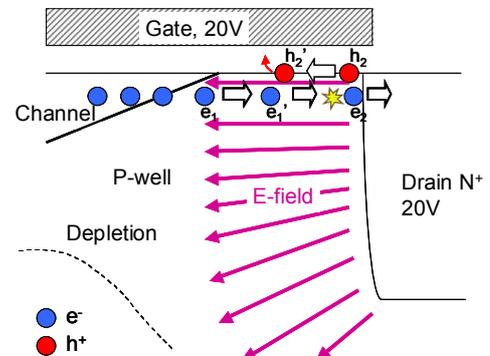
Fig. 7 Possible mechanism for hole trapping due to channel hot-electrons at high-drain-voltage stress condition.
