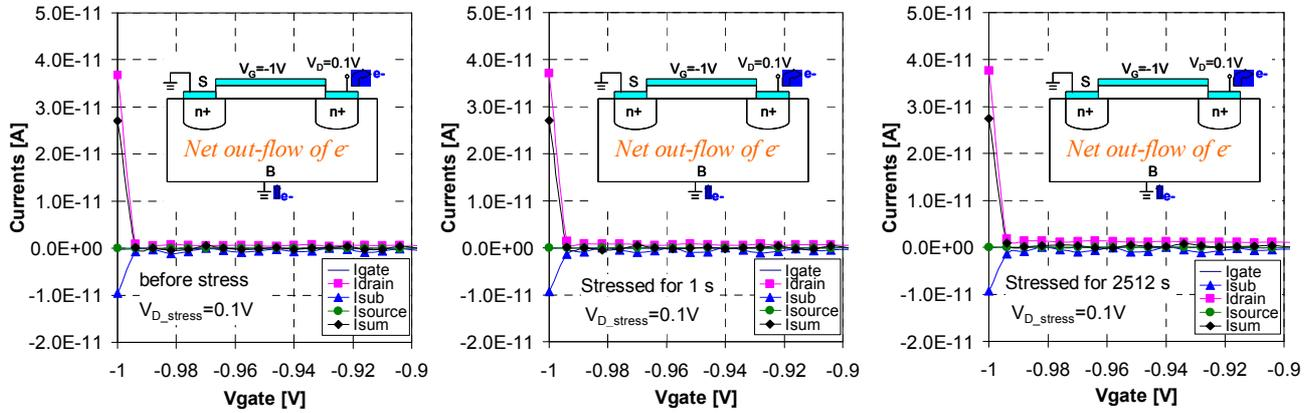
Fig. 5(a) Measurement of all the currents before stress for low-drain-voltage stress condition. The net current shows an out-flow of electrons.
