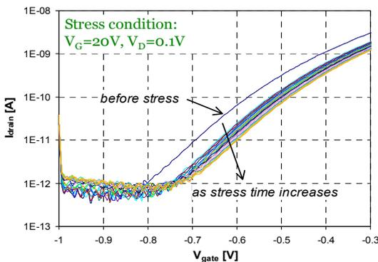
Fig. 3  $I_D$  versus  $V_G$  before stress and after stress as time increases in log scale (five curves per decade starting from 1 second). The stress condition is  $V_G = 20$  V and  $V_D = 0.1$  V.
