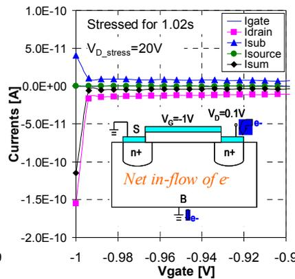
Fig. 4(b) Measurement of all the currents after short stress for high-drain-voltage stress condition. The net current shows an in-flow of electrons.
