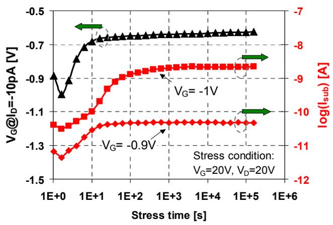
Fig. 6 Correlation, as a function of stress time, between the number of trapped holes, indicated by the gate voltage at which I<sub>D</sub> = -10 pA, and the junction leakage current between the drain and substrate (I<sub>sub</sub>). Stress condition used: V<sub>G</sub> = 20 V and V<sub>D</sub> = 20 V.
