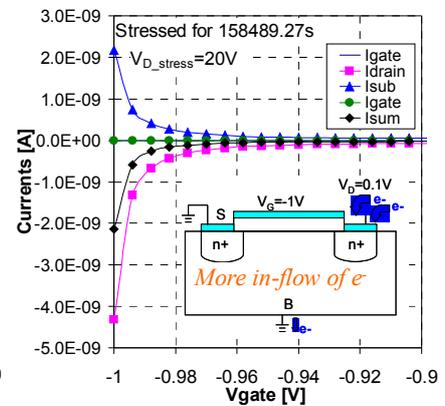
Fig. 4(c) Measurement of all the currents after long stress for high-drain-voltage stress condition. The net current shows more in-flow of electrons.
