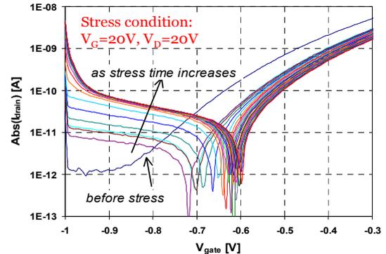
Fig. 2  $I_D$  versus  $V_G$  before stress and after stress as time increases in log scale (five curves per decade starting from 1 sec). The stress condition is  $V_G = 20$  V and  $V_D = 20$  V. The dips correspond to the sign change of the drain current.
