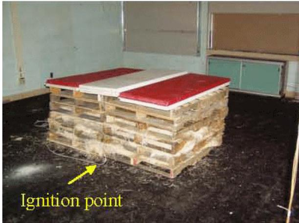
**Figure 2. Fuel package for classroom fires showing the wood pallets, excelsior, foam mats, and ignition point. The second ignition point is on the side opposite the ignition point shown in the figure.**
