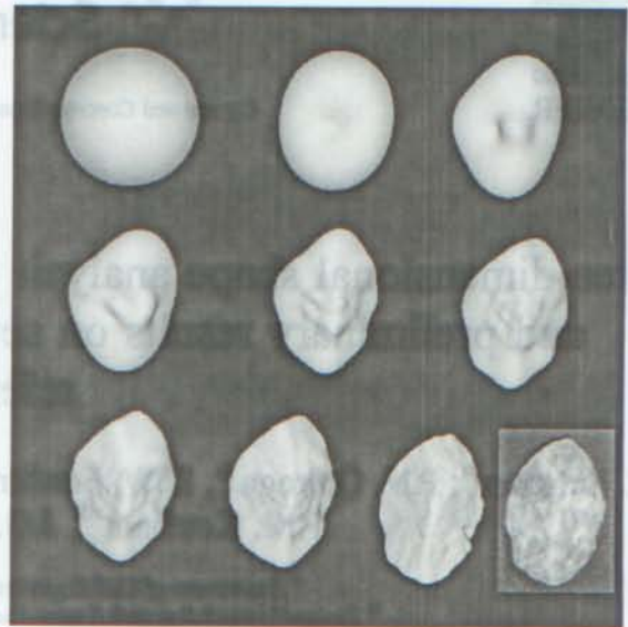
Fig. 1. This figure shows a series of 2-D images taken from the VRML particle reconstruction of reference rock 1. From top left to bottom right, the highest order of spherical harmonic coefficients used (value of N in Eq. (1)) was 0, 2, 4, 6, 9, 12, 15, 18, and 40. The final image on the bottom right is a digital camera image of the real rock, in the same orientation, about 80 mm in length in the vertical direction.
