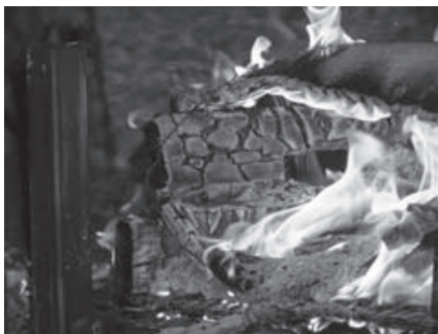
FIGURE 2.3.3 Charred Wood and a Charred Thermoset Plastic (Courtesy of National Institute of Standards and Technology)
