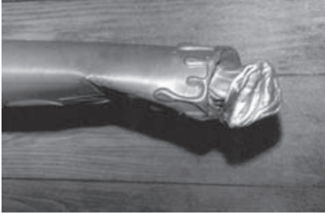
FIGURE 2.3.4 Melted Plastic (Source: Figure 4.11, User's Manual for NFPA 921 , 2005 edition, courtesy Jones and Bartlett Publishers)
