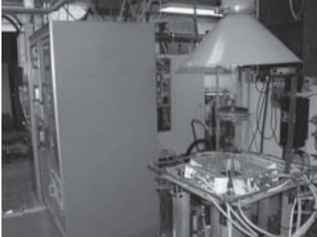
FIGURE 2.3.7 Quartz Heaters and Controlled Combustion Environment of the Fire Propagation Apparatus (Courtesy Ronald Alpert)
