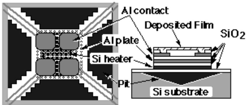
Figure I. Top: Scanning electron micrograph of a microhotplate. Bottom: Schematic top view (left) and side view (right) of the device.
