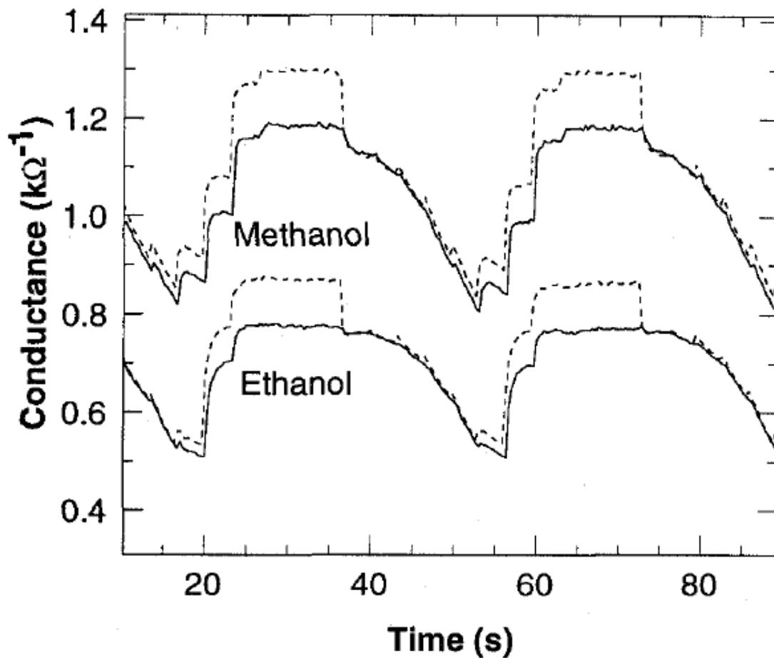
Figure 5. Conductance response to methanol and ethanol vapor (as labeled) during a temperature pulse sequence consisting of ten 100 ms pulses at each of 11 temperatures ranging from 20 °C to 520 °C. Solid and dashed curves are data collected 5 ms and 200 ms, respectively, after the pulse.
