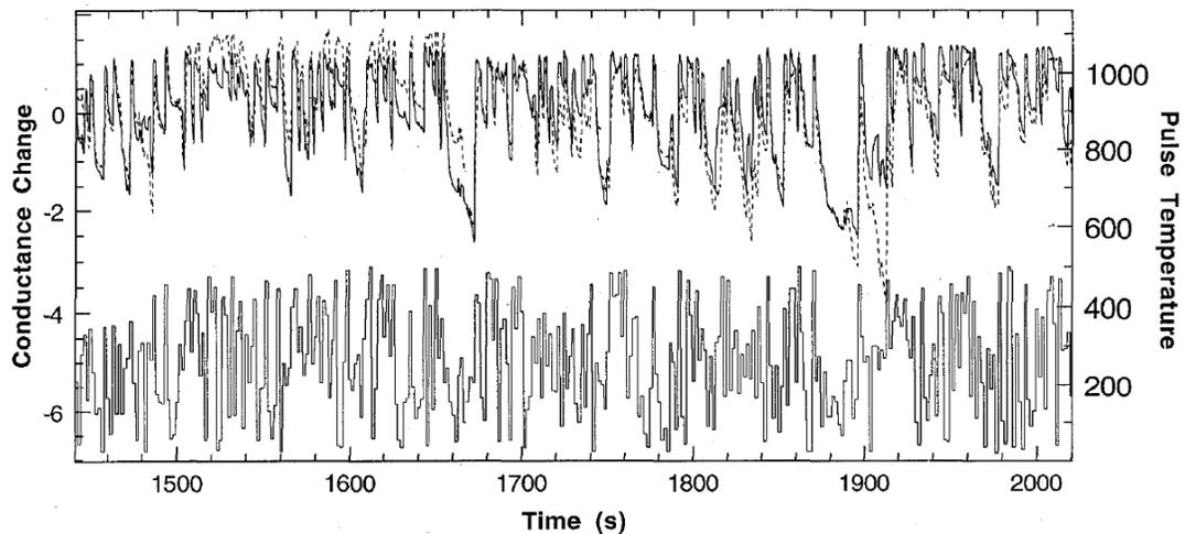
Figure 8. Normalized conductance change about the mean conductance during exposure to methanol (solid) and isopropanol (dashed) vapors during a long sequence of temperature pulses (lower trace). Larger response differences are seen near  $t = 1475$  and  $1925$  s.
