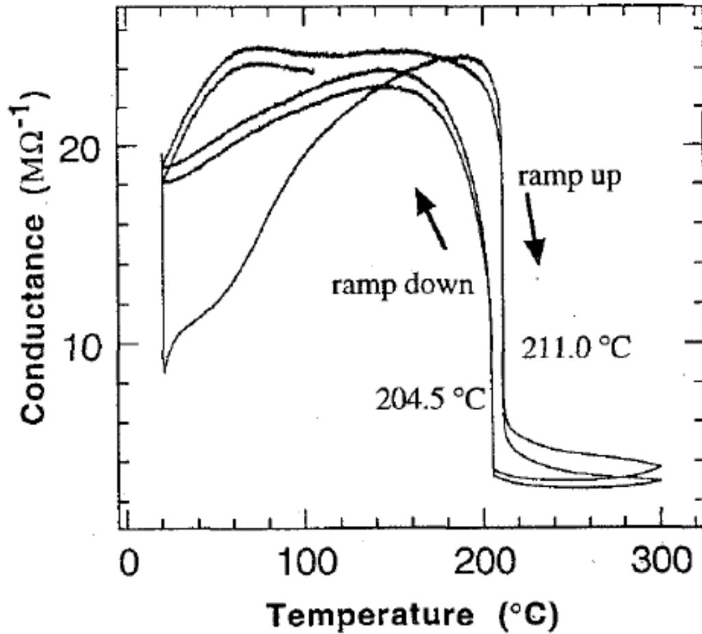
Figure. 7. Conductance as a function of temperature of a Pt-dosed SnO<sub>2</sub> film on a micro-hotplate in a concentration of 0.3% CO in air. The temperature was ramped between room temperature and 300°C at a rate of one cycle every 100 min.
