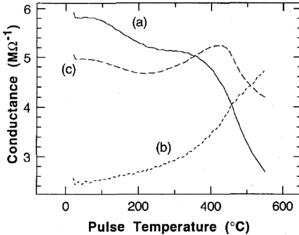
Figure 6. Response to a temperature pulse sequence consisting of 300 ms pulses ranging from 20 °C to 550 °C with a 5 °C temperature increment in the following test conditions: (a) 0.2 Pa O<sub>2</sub>, after heating in vacuum, (b) vacuum after treatment for curve (a), and (c) 0.5 Pa H<sub>2</sub>, after heating in vacuum.
