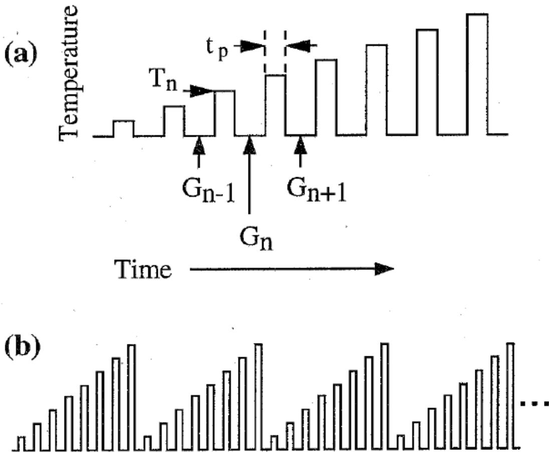
Figure 2. (a) Temperature pulse train applied to the micro-hotplate during sensor operation. Pulse width is  $t_p$ . Conductance  $G$  is measured between pulses, while the sample is at 20 °C. (b) Repetition of (a).
