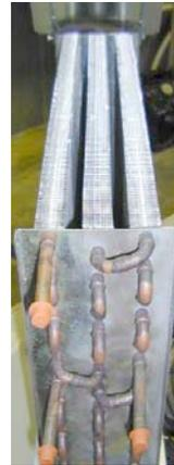
Figure 3. HX-slit-cut evaporator
