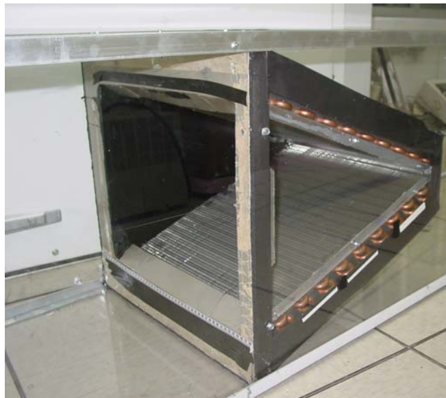
Figure 10. Test heat exchanger for PIV measurements.
