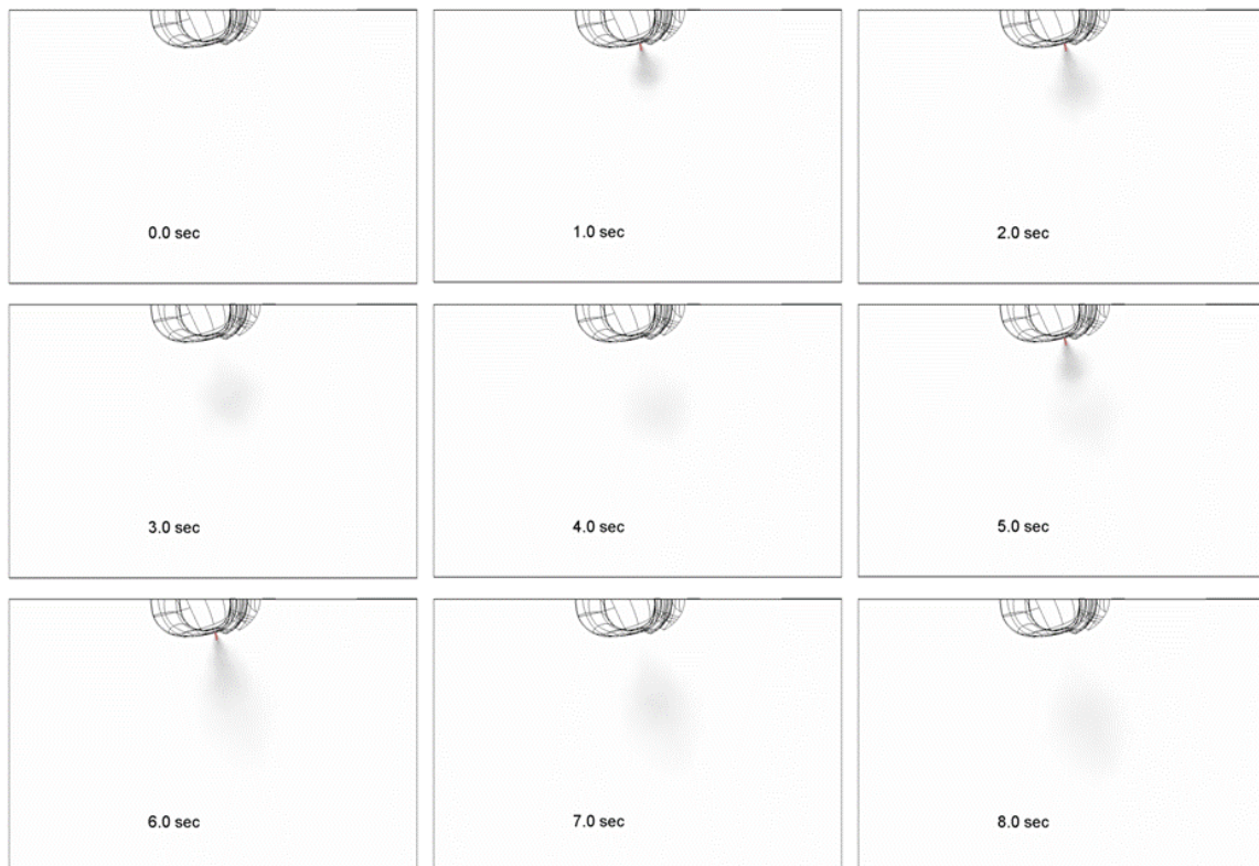
Figure 4. Time sequence of oxygen concentration from pure oxygen leak into pure propane environment.
