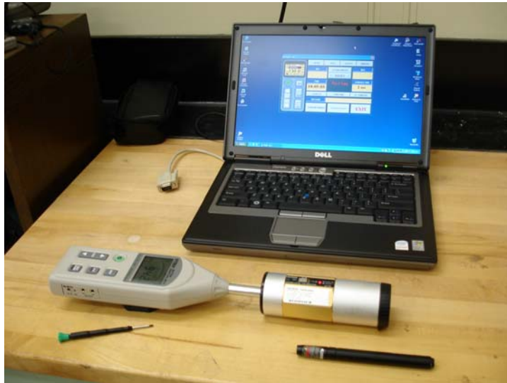
Figure 2. Photograph showing calibration of sound meter and laser used for alignment of sound meters and PASS devices.
