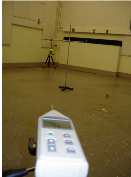
Figure 3. Photograph showing room and arrangement for unobstructed testing of stand alone PASS devices.
