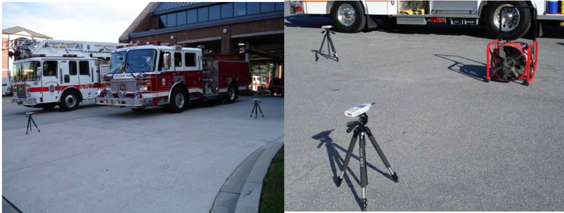
Figure 16. Photographs showing background sound level measurement tests.
