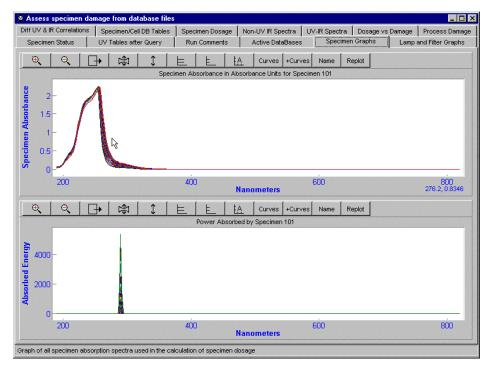
The specimen UV absorbance spectra are plotted on the "Specimen Graphs" page. The top plot is the series of specimen UV absorbances. Clearly, there was some change in the specimen, presumably as a result of damage. The bottom plot shows the dosage of the specimen - the amount of radiation remaining in the specimen.
