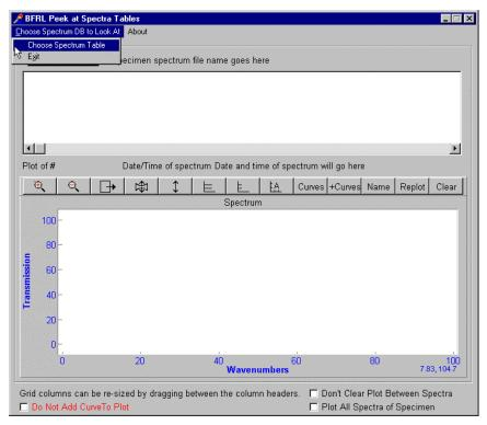
The file is read in using the "Choose Spectrum Table" menu item. Typed corrections can be made to the table parameters shown in the grid but not to the spectra.
