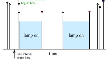
As shown below, the starting time of the exposure can be specified at any time before the exposures actually began, but it has to be adjusted to the time the lamp was first switched on.
