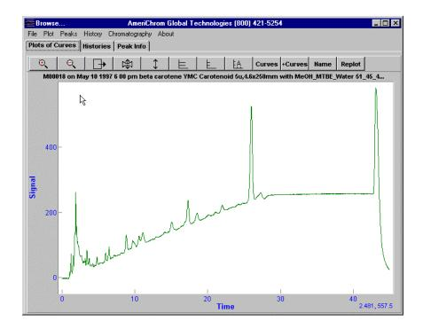
The first button is the zoom button. After the zoom button has been selected and is depressed, a rectangle can be drawn on the plot by dragging the mouse over the plot with the left mouse button down. When the mouse button is released, the contents of the rectangle will fill the screen, as shown in the next two figures.
