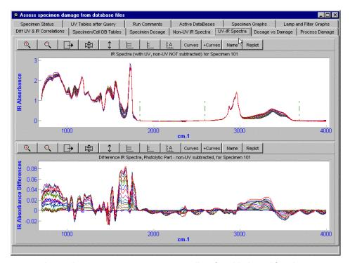
It may be necessary to measure or allow for ablation. After the program has read in the damage spectra, it calculates the apparent ablation for both the dark reaction, called control in the following figure, and for the UV degradation. The absorbance at the ablation site (specified on the "Process Damage" page) is used to estimate the sample thickness and hence the ablation.
