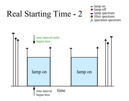
Depending on where the user wants to begin the calculations, there are other possibilities to consider. If the time the user specified was "inside" an exposure interval, that time must be maintained.
