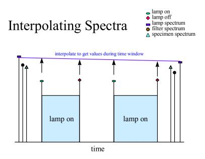
First, there are no spectra between the two sets of lamp-on times. Therefore, the spectra will be interpolated across the time interval to assess the values they would have had if they had been taken at the time in the middle of the figure.
