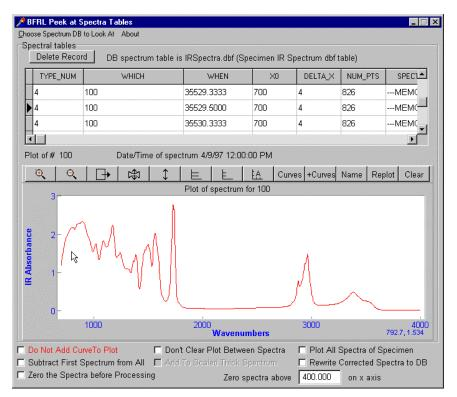
A record can be selected using the grid cursor at the left hand side of the grid or by clicking on the scroll bar at the right hand side of the grid.
