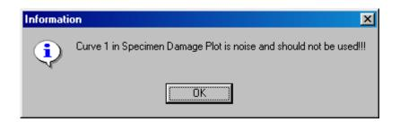
because the damage/time plot, the top plot in the next figure, is too noisy, i.e., the line contains too many reversals in sign of the slope.
