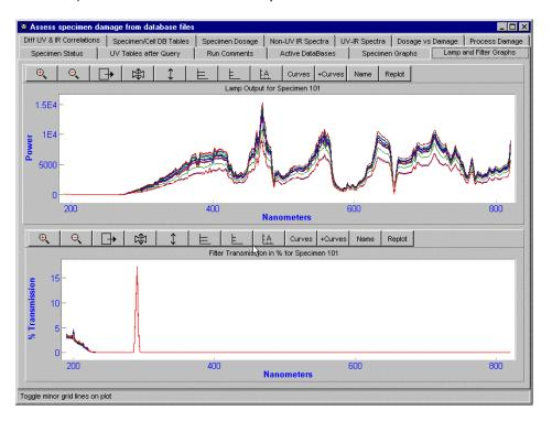
2) the filter was a narrow band-pass filter centered at about 300 nm.
