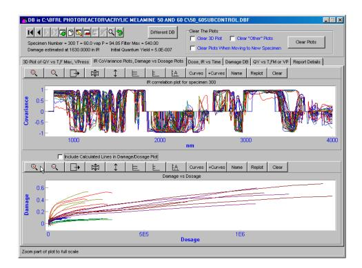
The plot was zoomed (using the first plot button) and the short lines identified using the plot "Names" button. As shown, one of the short lines is for the wavelength of 290 nm.
