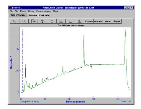
After some lines have been drawn (presumably at least two), segments between vertical lines should be drawn to see how well the segments follow the curve and hence to see if enough vertical lines have been drawn to allow a reasonable subtraction of the slope in the curve. Select the "Draw segments between vertical lines" option in the dialog box.
