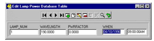
The UV-visible spectra currently cover the wavelength range 190 to 820 nanometers. A lamp power factor must be supplied for each of the wavelengths to convert the lamp intensity readings into watts. The lamp output factor at 190 nm is 0. Non-zero lamp output begins at about 270 nm.
