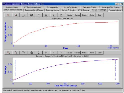
The program now has dosage vs. time and damage vs. time, so it can easily calculate damage vs. dosage, using the time axis as a common
