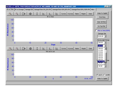
If plots are desired of damage versus temperature interpolated to various levels of humidity (currently fixed at 0%, 20%, 40%, 60%, 80% and 100%), the box "Plot vs Time [RH%]"should be checked.
