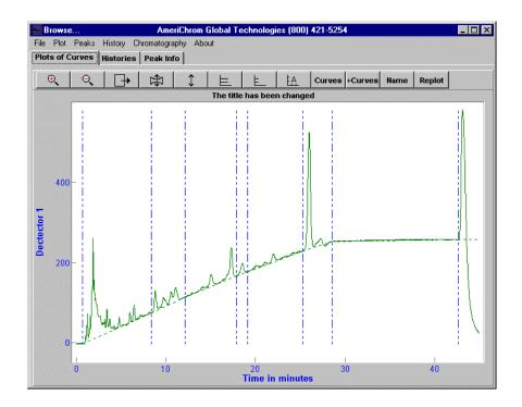
This is now satisfactory and we can subtract the line segments from the original curve to remove the effect of the slope. We bring up the dialog, select "Baseline defined between vertical lines", click on OK, and have the result:
