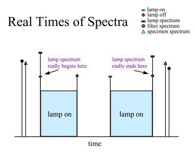
However, it is not quite that simple. There was no photolytic exposure of the specimen while the lamp was off so the time to use for the lamp spectrum is when the lamp was actually switched on and off, not the times the spectra were measured.
