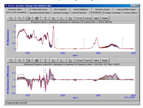
For example, a specimen was processed manually, the dosage was integrated, and the difference damage plot was right-clicked in two places, shown by vertical lines in the next figure.
