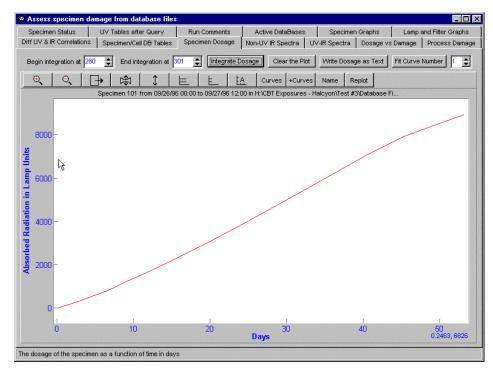
After the filter width limits have been chosen, clicking on the "Integrate Dosage" button puts a new curve in the dosage/time plot. If more than one curve is in the plot, the curve to use to estimate dosage as a function of time can be set using the spin button "Fit Curve Number" in the top right hand corner of the page. The dosage/time curve must be filled in before damage sites can be selected in the damage plots.
