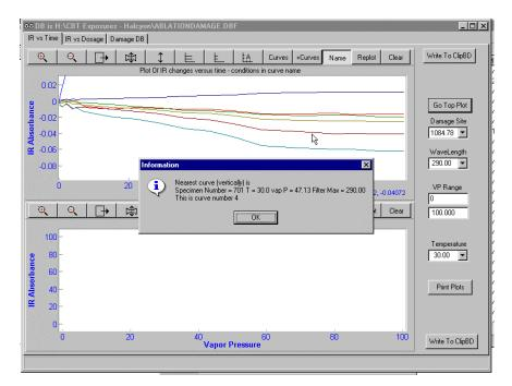
When the plot is not in names mode, right clicking puts a new line in the bottom plot. The line is the damage as a function of vapor pressure at the time clicked in the top plot. This line covers all curves in the top plot. (Curves are added to the top plot each time the "Go Top Plot" button is clicked. The plot is cleared using the "Clear" button over the plot.)
