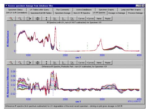
If the mouse is right-clicked on the difference UV-exposed specimens plot (or the top IR plot), the IR absorbances at the point clicked in each of the spectra are plotted as a function of time (the time at which each spectrum was taken) in the top plot on the "Dosage Vs Damage" page (see the next figure).
