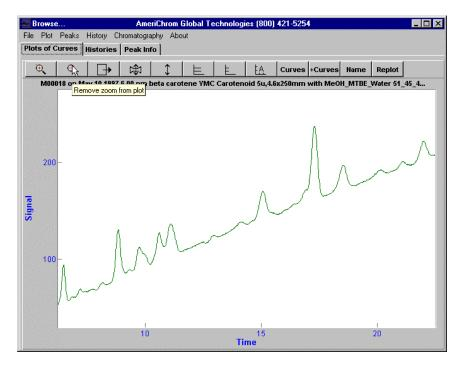
When the plot has been zoomed, the plot contents can be dragged around by first clicking on the third plot button, as indicated below, then dragging the plot contents with the left mouse button depressed. In this way, new areas can be scrolled into the visible area from out of the picture, as shown in the next two figures. The numbers on the horizontal axis show that the curve has been dragged from left to right.
