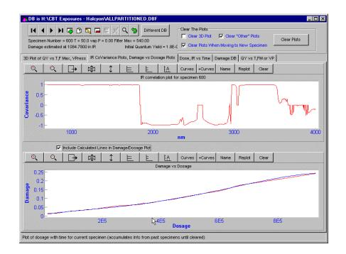
The bottom plot is the damage dosage relationship. The quantum yield is the slope of curve in the bottom plot. The red line in the bottom plot is the observed damage/dosage relationship, the blue curve is the fitted polynomial. (These lines are only red and blue when they are the first and second curves in the plot. Curves added later have contrasting colors.)
