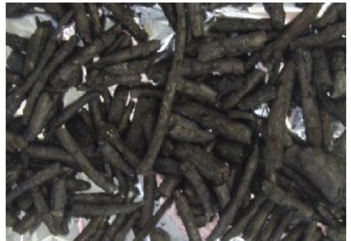
Fig. 3. Digital photograph showing typical firebrands collected when 8 mm diameter, 50 mm long cylinders were used.
