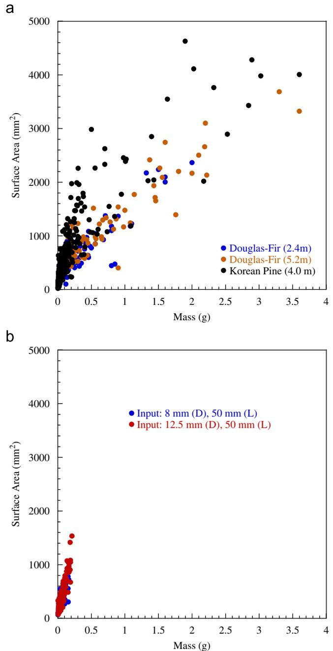
Fig. 8. (a) Calculated surface area plotted as a function of mass for firebrands produced from burning trees. (b) Calculated surface area plotted as a function of mass for firebrands produced from the firebrand generator.
