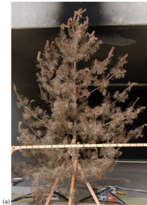
Figure 1. (a) A photograph of Korean pine ( Pinus koraiensis ) tree used for the firebrand collection experiments, MC=13% and (b) a drawing of the hexagonal burner used to ignite the Korean pine and Douglas-fir trees.
