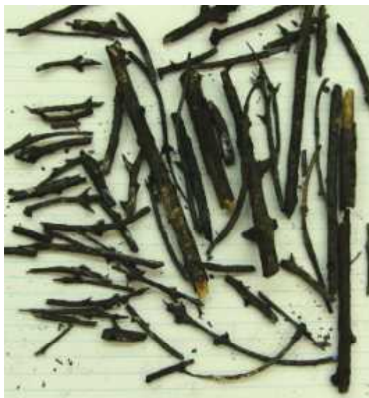
Fig. 2 Digital photographs showing samples of the firebrands collected as a function of tree size and moisture content. Tree Height 5.2 m, Moisture Content 20 %.
