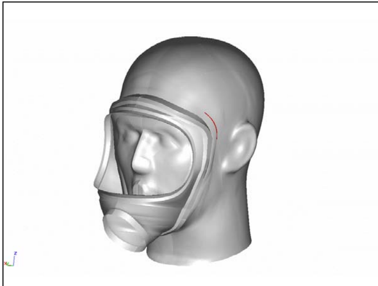
Figure 2. Model geometry for headform combined with respirator facepiece. Red mark indicates a possible location for a leak.
