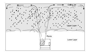
plume does not truly mix with the upper layer initially as indicated in the figure
