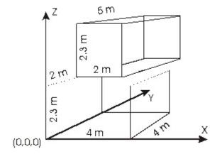
compartment is at the station elevation and the second is 2.3 m above the first. The configuration would be used, for example, to build a two floor structure. The position of the front, lower corner of compartment 2 is at (0.0 m, 2.0 m, 2.3 m).
