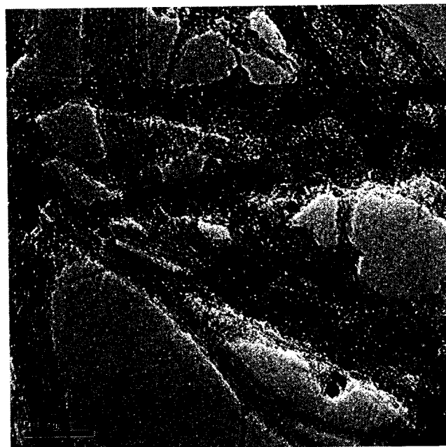
Fig. 15. TEM image of the bottom layer of the residue of PMMA/SWNT(0.5%) collected after the gasification test.
