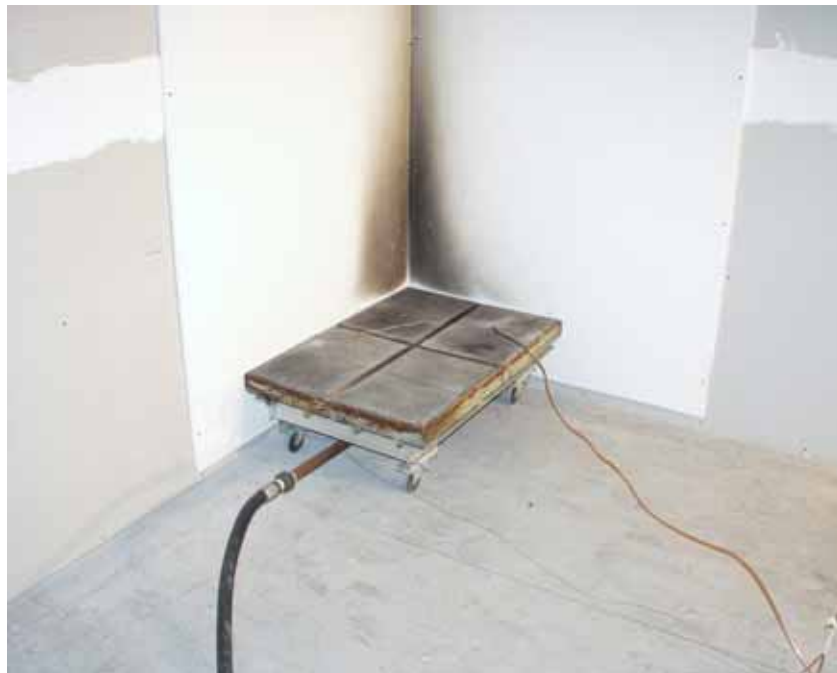
Figure 8 Gas burner placed for a corner experiment.
