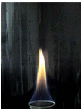
**Figure 1** A video image of a methane cup-burner flame in air.  $U_{\text{CH}_4} = 0.92$  cm/s,  $U_{\text{ox}} = 10.7$  cm/s.
