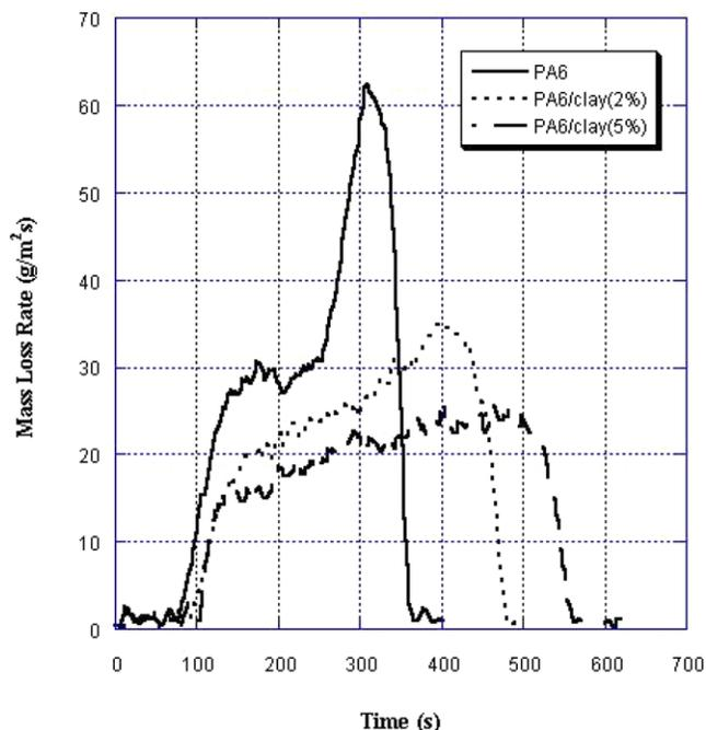
Fig. 4. Effects of clay content on mass burning rate of PA6 (8 mm thick) at 50 kW/m<sup>2</sup>.
