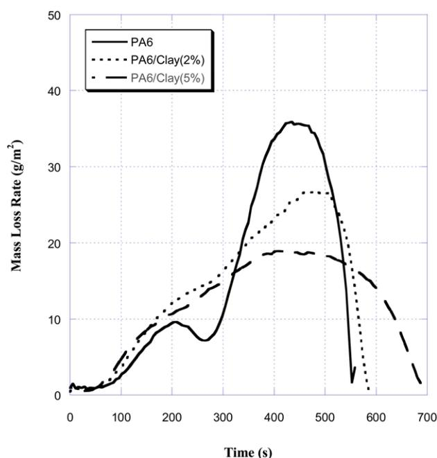
Fig. 5. Effects of clay content on mass loss rate of PA6 (8 mm thick) in N<sub>2</sub> at 50 kW/m<sup>2</sup>.
