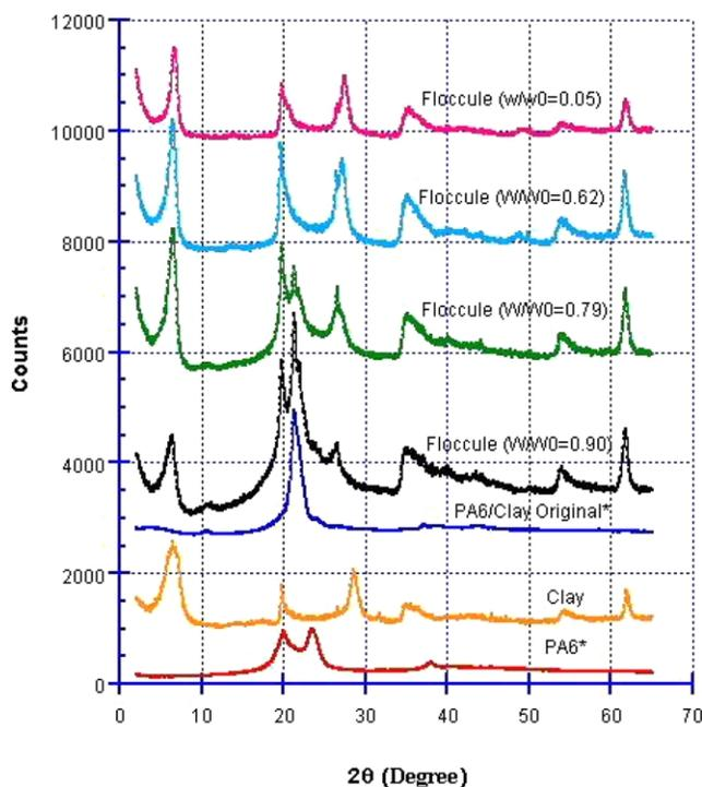
Fig. 13. XRD of PA6, Clay, PA6/Clay(5%), and carbonaceous floccules collected at various fractions of sample mass loss at  $50 \text{ kW/m}^2$  in  $\text{N}_2$ . \*PA6 and PA6/Clay original values reduced to 10% of measured values.
