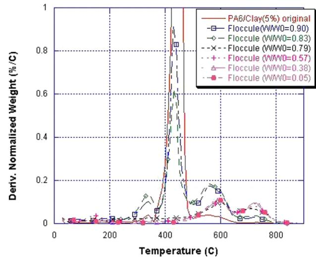
Fig. 10. DTG plot of carbonaceous floccules of PA6/Clay(5%) collected at various sample mass losses at external flux of 50 kW/m<sup>2</sup> in N<sub>2</sub>.
