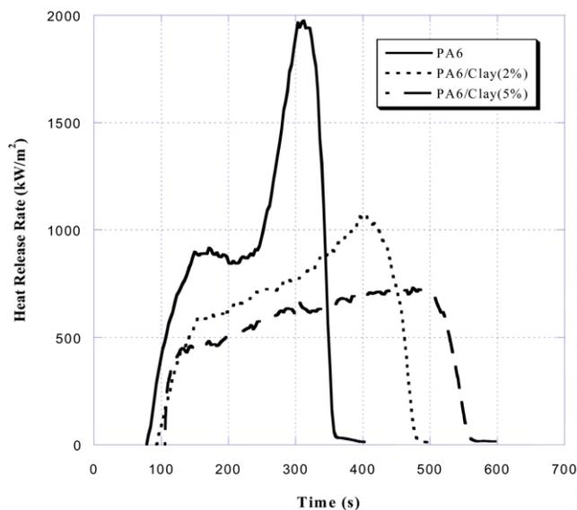
Fig. 3. Effects of clay content on heat release rate of PA6 (8 mm thick) at 50 kW/m<sup>2</sup>.
