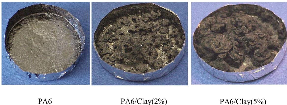
Fig. 7. Residue pictures at the end of the gasification tests in N<sub>2</sub> at 50 kW/m<sup>2</sup>.
