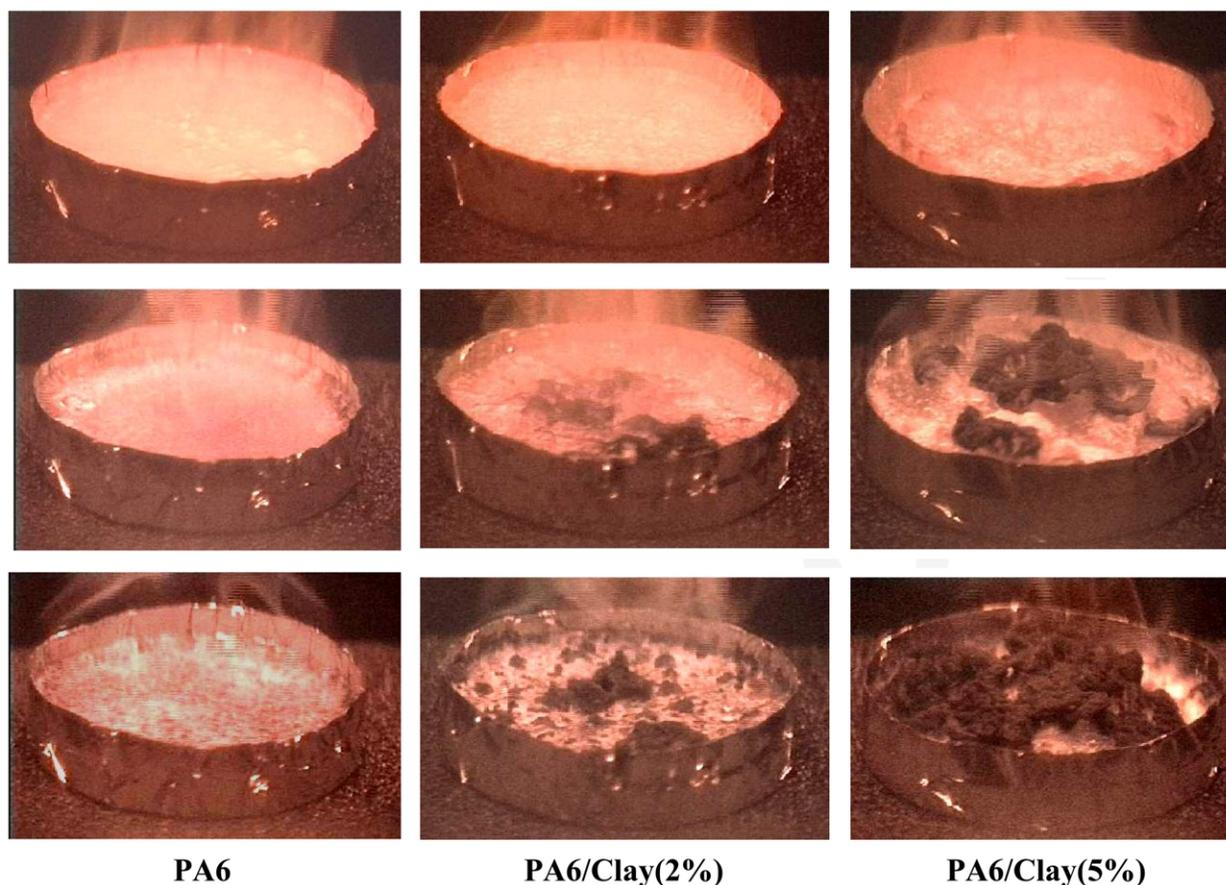
Fig. 6. Selected video images at 100, 200, and 400 s in nitrogen at 50 kW/m<sup>2</sup>.
