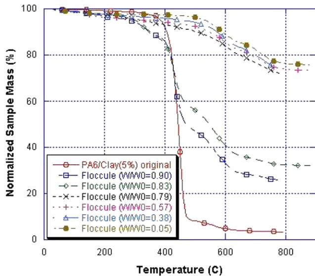
Fig. 9. TGA of carbonaceous floccules of PA6/Clay(5%), collected at various sample losses at external flux of 50 kW/m<sup>2</sup> in N<sub>2</sub> under air at heating rate of 10 °C/min.
