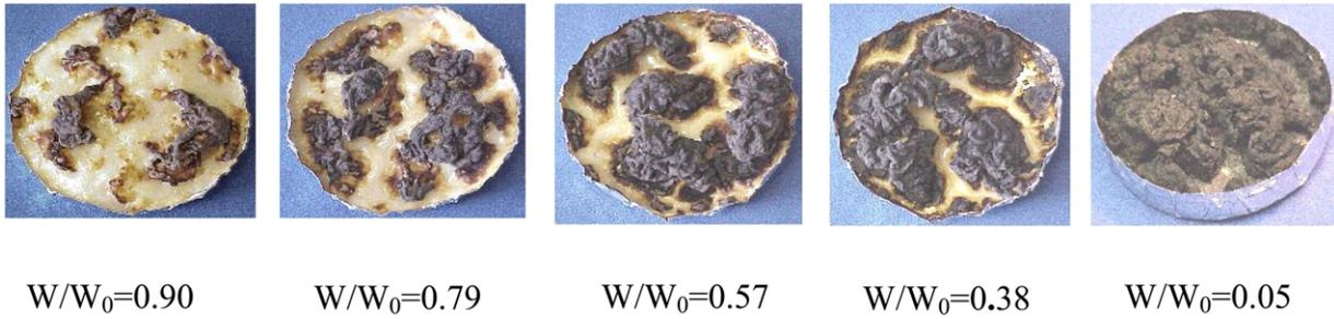
Fig. 8. Pictures of the residues of PA6/Clay(5%) collected when it lost various fractions of its mass in a nitrogen atmosphere at 50 kW/m<sup>2</sup>.
