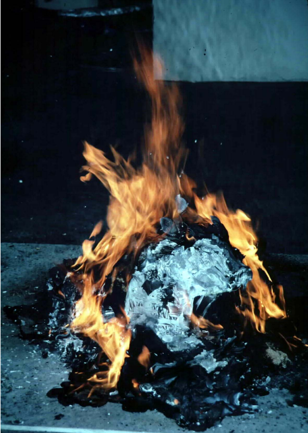
Figure 14. Trash Container 2 melts and opens exposing burning debris pile.
