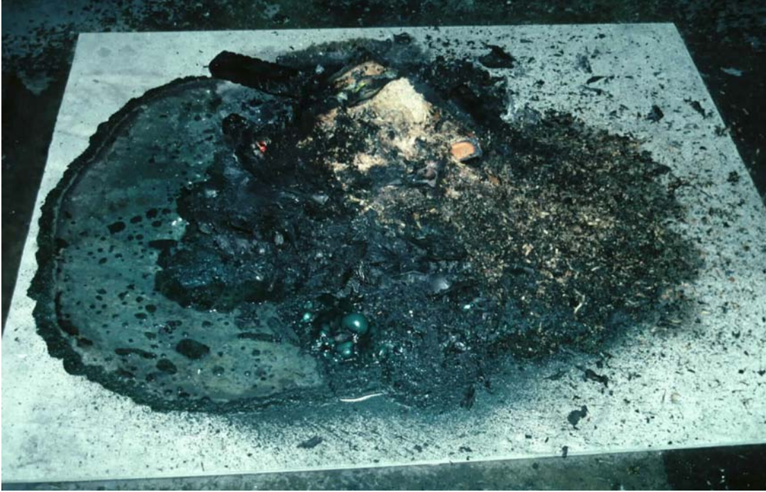
Figure 9. Remains of Trash Container 1 after test.
