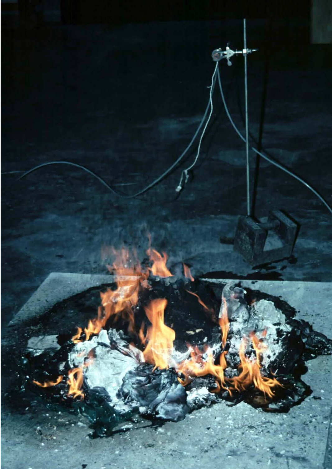
Figure 15. Remains of Trash Container 2 just prior to suppression at 900 s.
