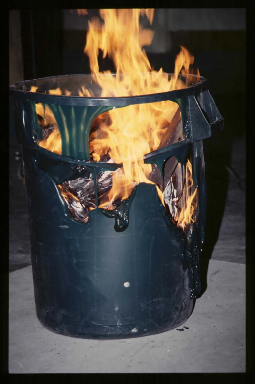
Figure 5. Trash Container 1 melting and allowing more ventilation for the burning fuel it contains.
