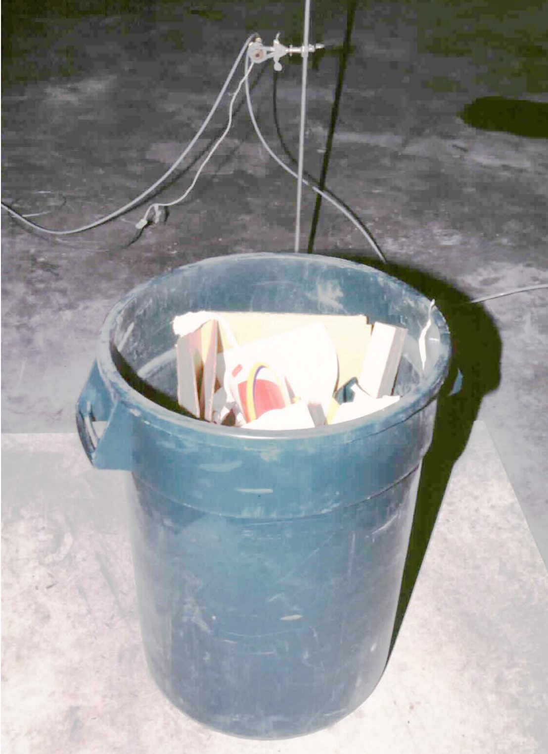
Figure 1. Loaded Trash Container prior to ignition.
