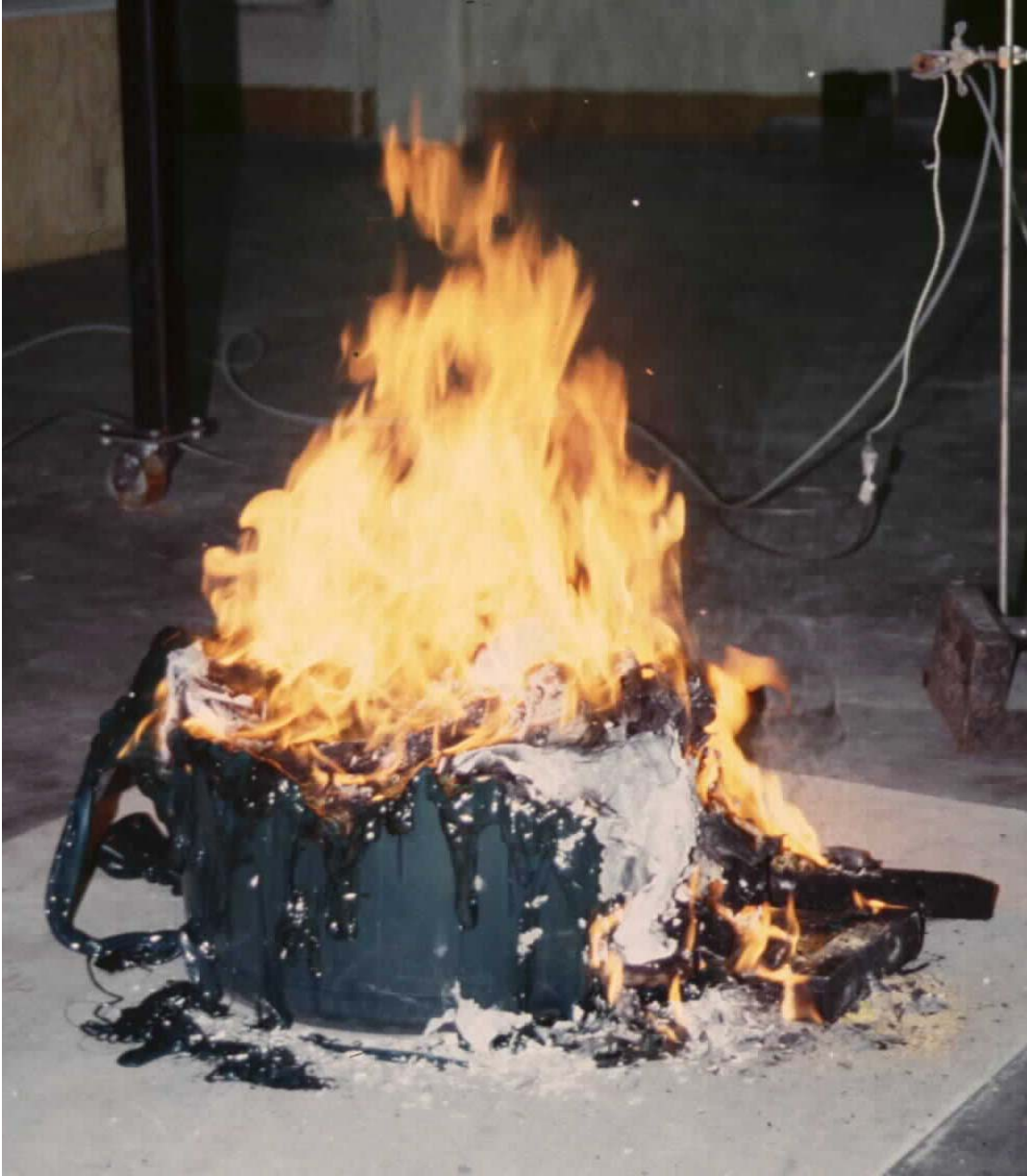
Figure 7. Upper portion of container melts and collapses.
