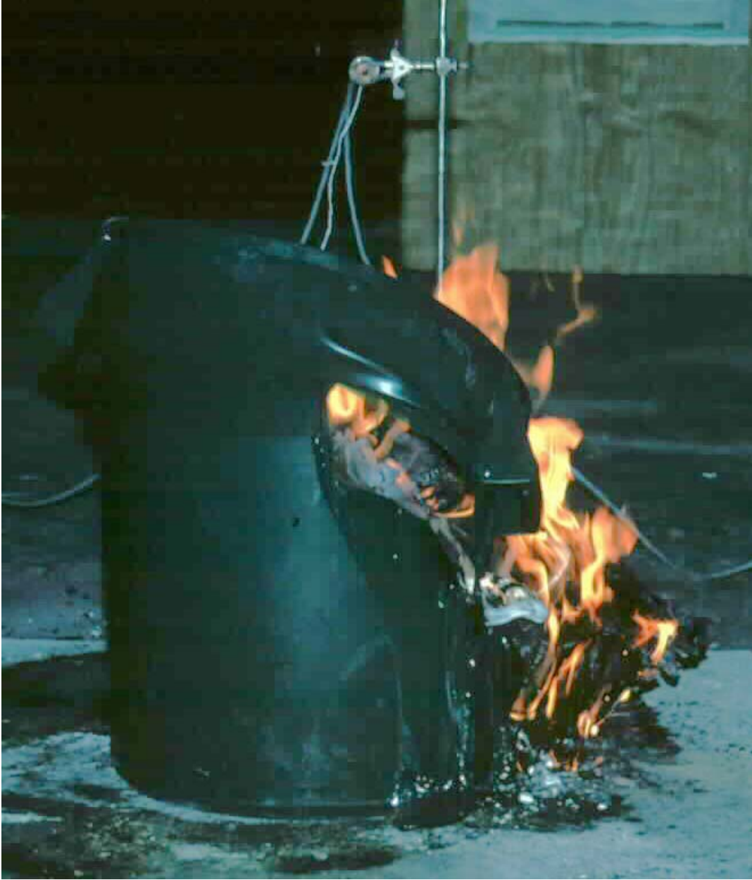
Figure 13. Trash Container 2 collapses in on itself, obstructing ventilation and limiting fire growth.
