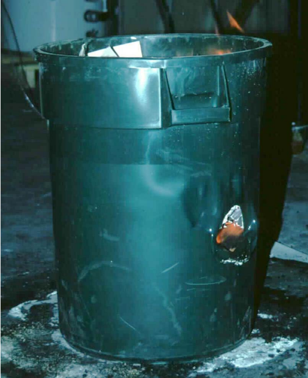
Figure 11. A hole opens in the side of Trash Container 2 near the point of ignition.
