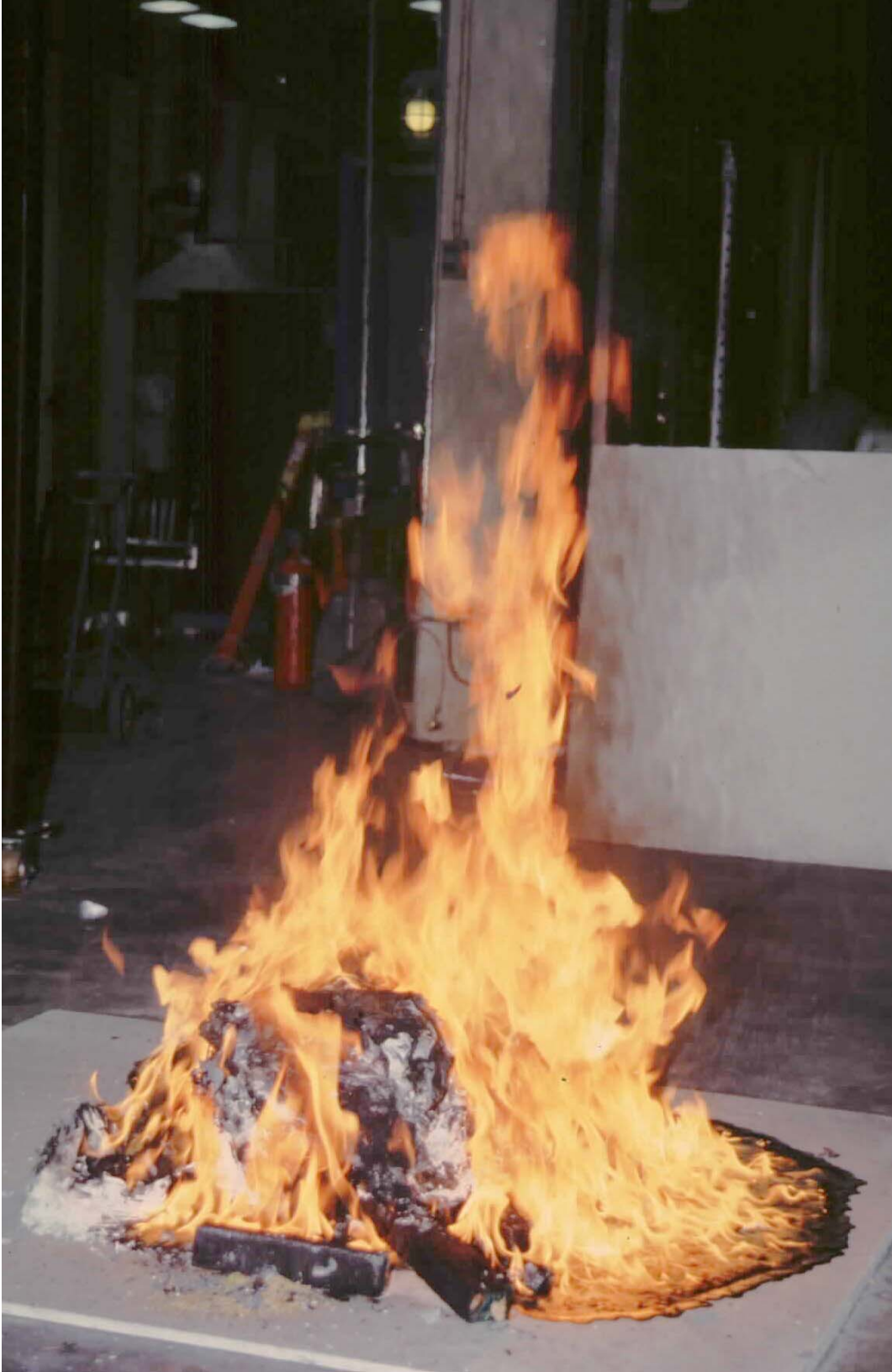
Figure 8. Molten plastic burning around debris pile.
