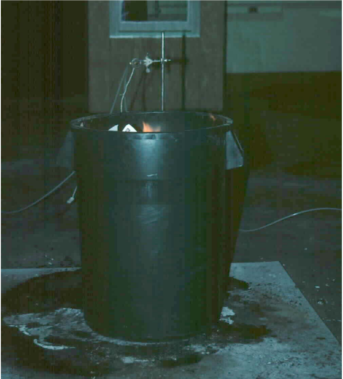
Figure 10. Trash Container 2 just after ignition.
