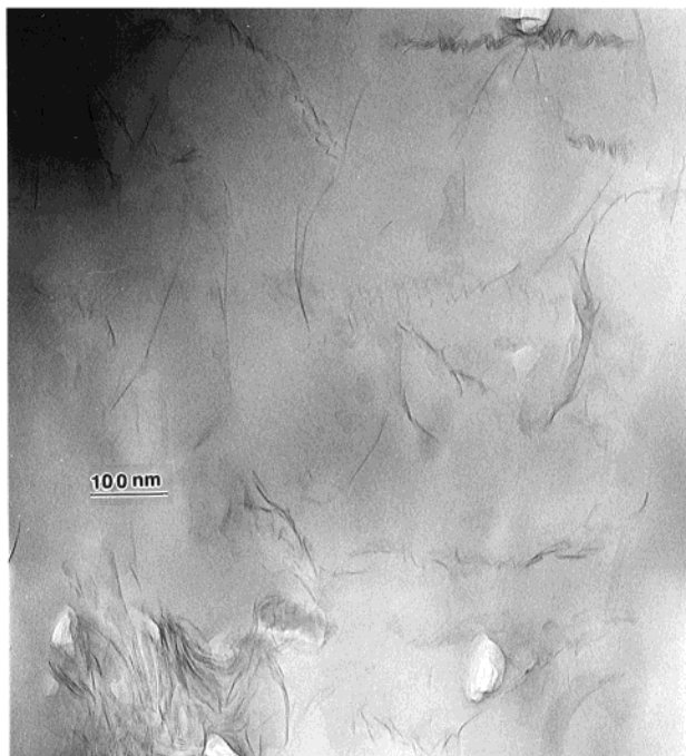
Figure 9. TEM image of DMHDIM-MMT/PS (95:5) prepared by solution blending with sonication.
