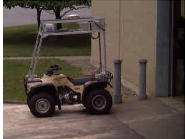
Figure 2. Photograph of the instrumented All-Terrain Vehicle. The top layer of the frame supports the first GPS antenna (for position), the lower level houses the real-time computer, wireless Ethernet, compass and GPS receiver. The Scanning LADAR will be mounted forwardmost on the top deck.
