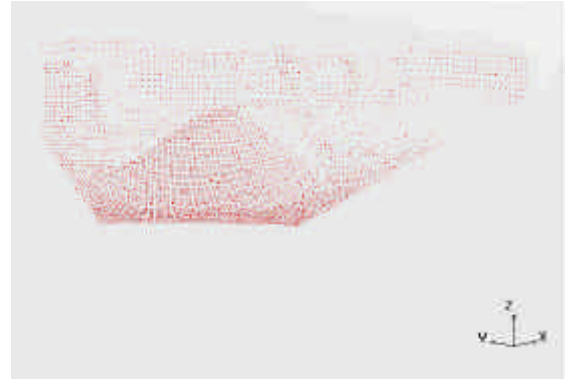
Figure 3. One LADAR scan of a simple piece of terrain, a pile of sand. Several such views, from known locations can be merged to form a simple model of the surface.
