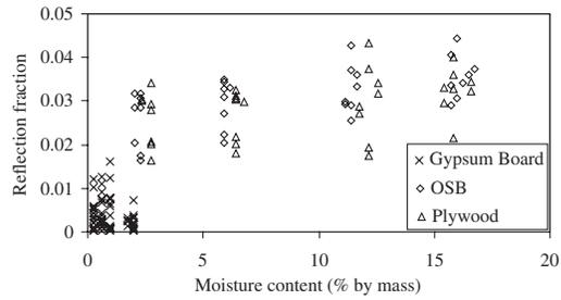
Figure 8. Reflection fractions for 3 different materials. Antenna placed on exterior (sheathing) side of assembly.
