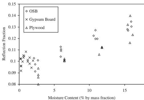
Figure 4. Reflection fraction vs. moisture content.
