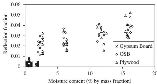
Figure 7. Reflection fractions for 3 different materials. Antenna placed on interior (gypsum) side of assembly.
