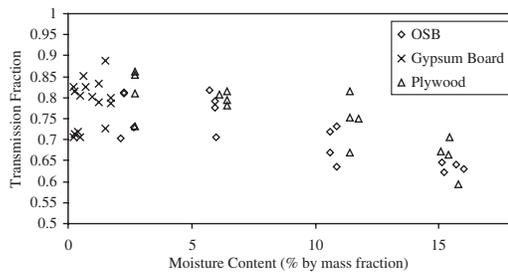
Figure 5. Transmission fraction vs. moisture content.
