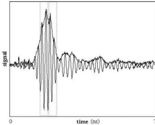
Figure 6. Sample waveform with the magnitude of its Hilbert transform and sample time frames used to compute reflections from each panel.
