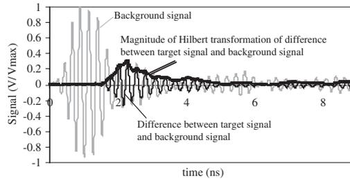
Figure 2. Typical set of waveforms used in analysis.
