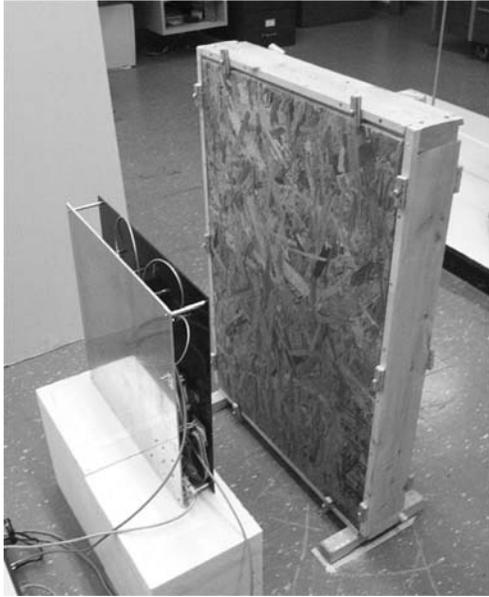
Figure 1. OSB specimen (right) and antenna holder (left).
