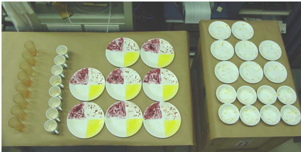
Figure 5: Photograph of soiled dishware used for testing two dishwashers
