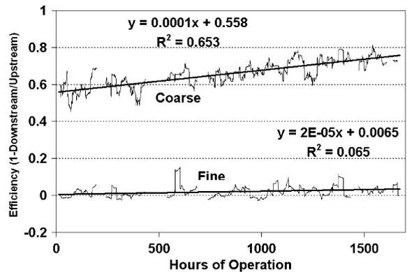
Fig. 3. Volume-weighted 12-h average single-pass efficiency of mechanical filter (MECH) for fine (0.3–2.5  $\mu\text{m}$ ) and coarse (2.5–10  $\mu\text{m}$ ) particles. The filter was not cleaned over the 2 months of operation.
