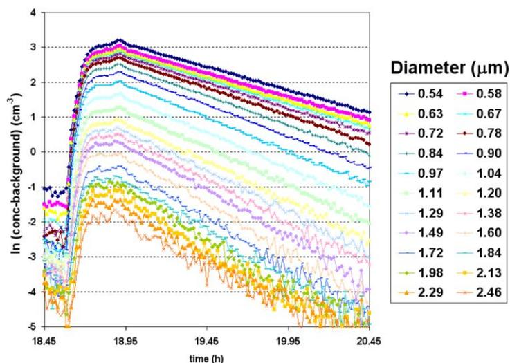
Fig. 1. Decay of fine particles ( $<2.5\ \mu\text{m}$ ) in basement as measured by APS after cooking tortillas in kitchen. Successive points are 1 min apart.
