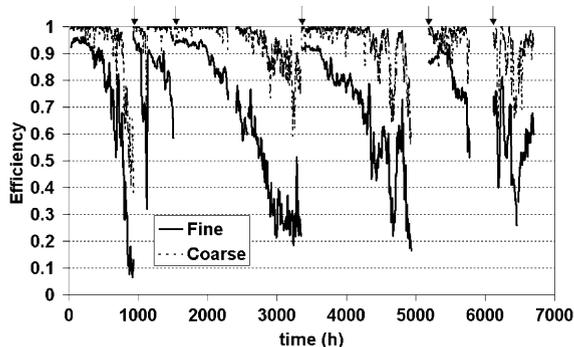
Fig. 2. Volume-weighted 12-h average single-pass efficiency of ESP for fine particles (between 0.3 and 2.5  $\mu\text{m}$ ) and coarse particles (2.5–10  $\mu\text{m}$ ) as a function of time since cleaning. Arrows mark five cleaning episodes that occurred during the 9 months of testing.
