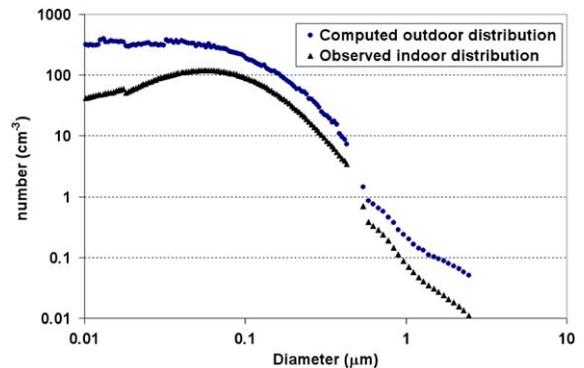
Fig. 6. Computed outdoor distribution of particles based on observed indoor distribution over the year 2000 ( $N = 45,000$  measurements), using the calculated size-specific deposition rates for the fan-on no-filter condition.
