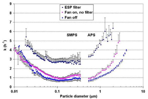
Fig. 5. Deposition rates with error bars showing either +1 SE or -1 SE (only three of four cases shown for clarity).
