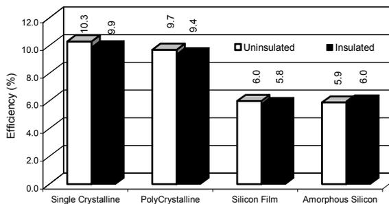
Figure 2 Overall BIPV Conversion Efficiency
