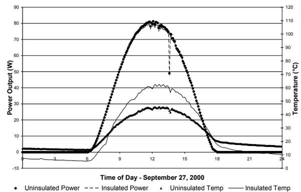
Figure 4 Amorphous Silicon Power Output and Temperature: Uninsulated Versus Insulated
